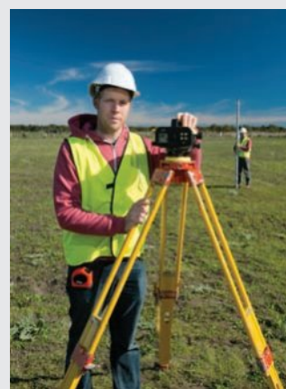
Land surveyors measure the horizontal and vertical distance between two locations of different altitudes. The straight line distance of the slope, which forms a hypotenuse, is calculated using Pythagoras' theorem.
