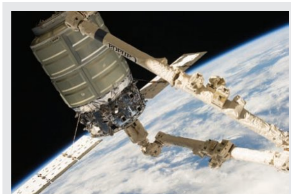
The International Space Station has a 16.94 m robotic arm with four segments that is used on spacewalks, and for capturing and releasing visiting spacecraft. Trigonometry is used to calculate the required angle between segments for grappling specific spacecraft.
