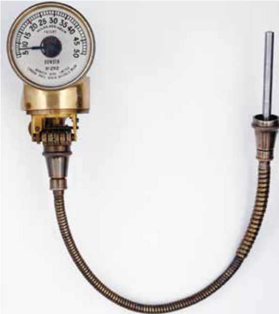
FIGURE 8.14 An older speedometer with a rotating magnet to help detect speed
