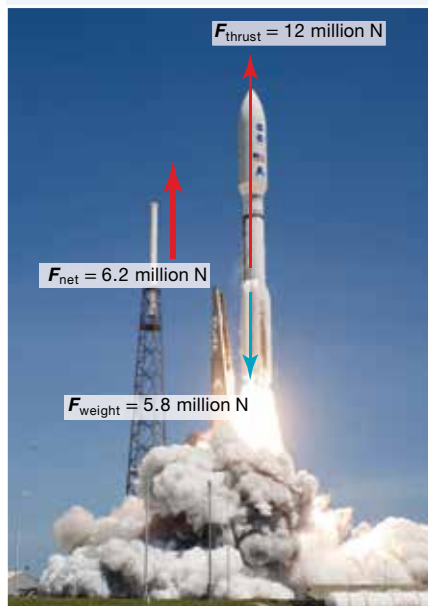
FIGURE 8.24 A spacecraft is launched by powerful rockets — yet it seems to take a long time to get off the ground. Newton's Second Law provides an explanation.
