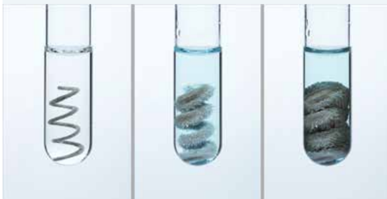
FIGURE 4.45 Production of silver crystals by a displacement reaction between copper atoms and silver ions
