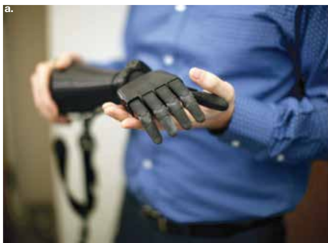
FIGURE 5.44 a. A prosthetic limb for amputees made from using a 3D-printer and polylactic acid; b. a bioware plastic tumbler made from polylactic acid that will compost within six days
