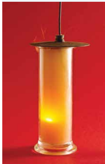
FIGURE 5.12 Sodium burns in chlorine to form sodium chloride
