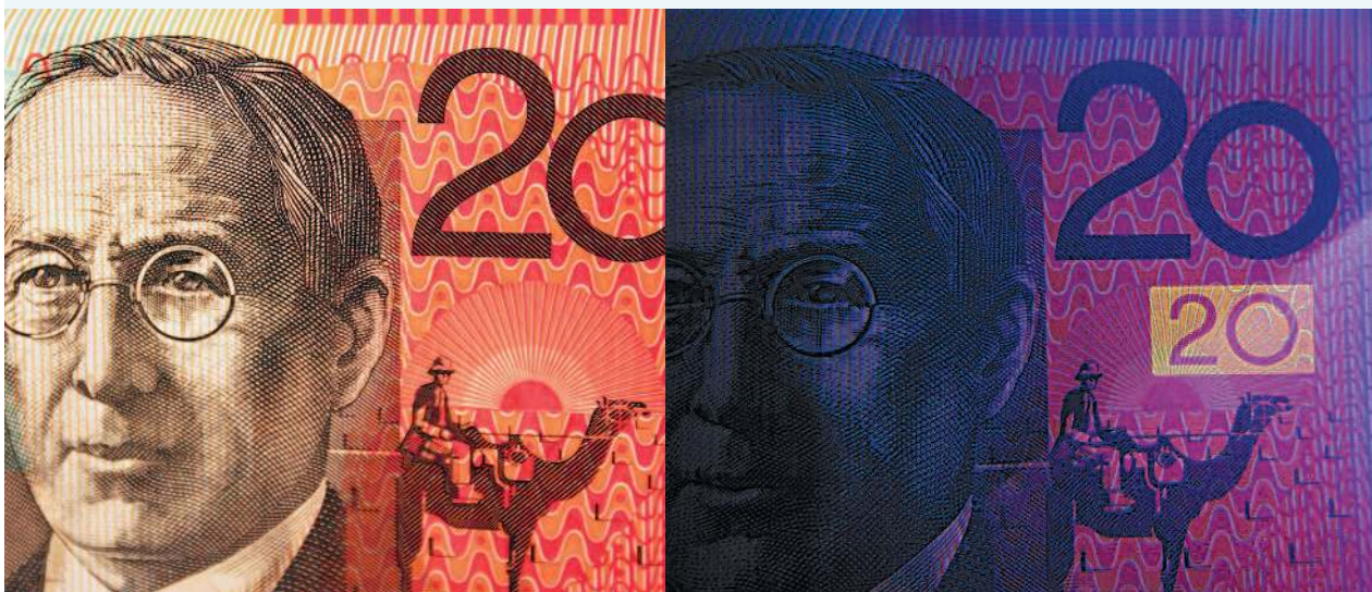
FIGURE 11.19 UV light can be used to explore counterfeit money. This twenty dollar note is genuine as you can see the feature fluoresce under the UV light.
