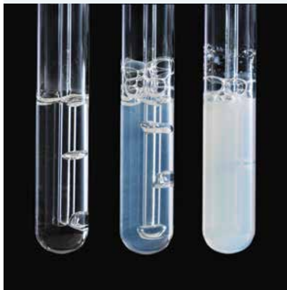
FIGURE 5.14 Bubbling carbon dioxide gas through lime water turns the solution cloudy
