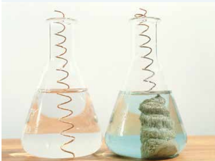
FIGURE 5.17 Copper displacing silver from silver nitrate
