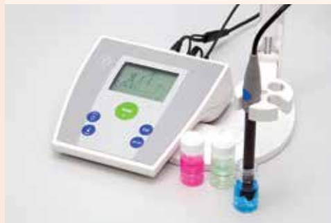
FIGURE 1.32 A pH meter needs to be calibrated regularly to ensure it gives accurate readings.
