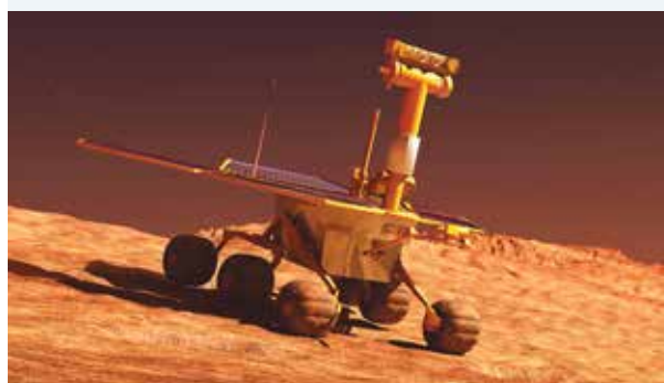
FIGURE 9.57 An example of a Mars rover, which shows the multi-panel solar array spread out like wings
