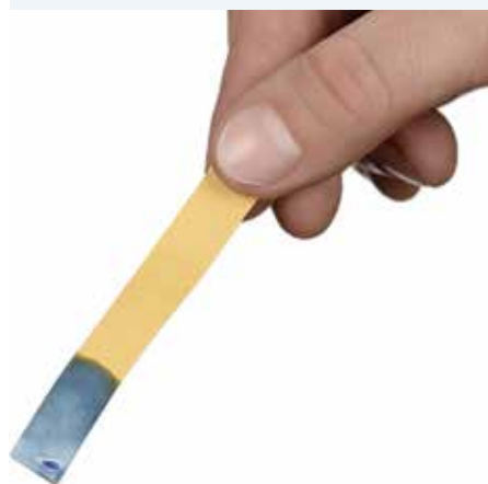
FIGURE 5.20 Universal Indicator paper turns blue when dipped into a basic solution.
