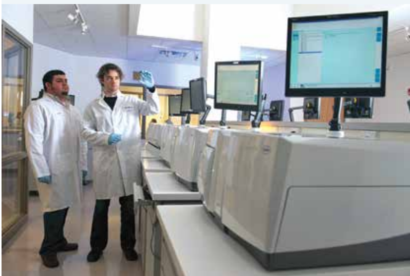
FIGURE 2.63 A DNA sequencing machine. These machines are capable of processing huge numbers of DNA sequences. One machine can sequence 400 to 600 million bases over a ten-hour run.
