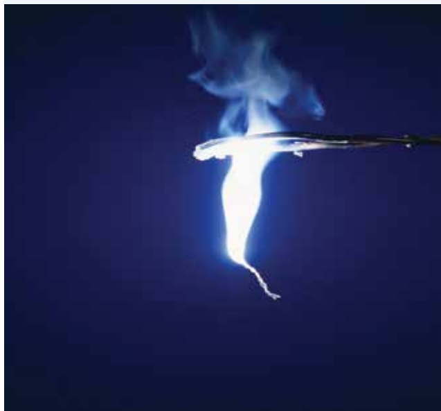
FIGURE 5.9 Magnesium ribbon burning in air with a brilliant white light
