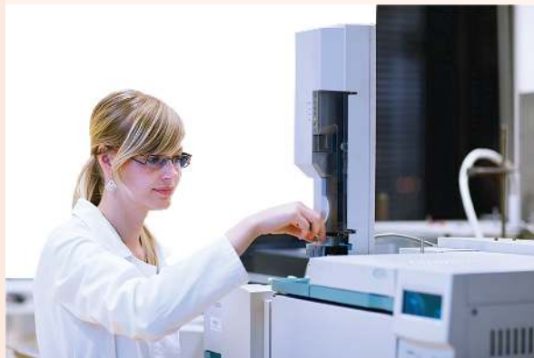
FIGURE 6.22 A high-performance liquid chromatography (HPLC) machine automatically separates mixtures by chromatography.
