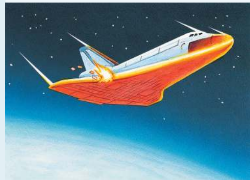
FIGURE 8.20 Damage to Columbia 's ceramic tiles is believed to have caused it to overheat and explode on re-entry in a tragic incident in 2003.
