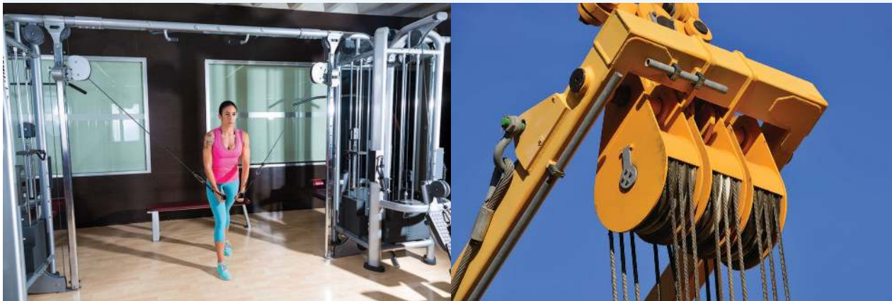
FIGURE 8.62 A pulley changes the direction the effort is needed to lift a load, making it easier.
