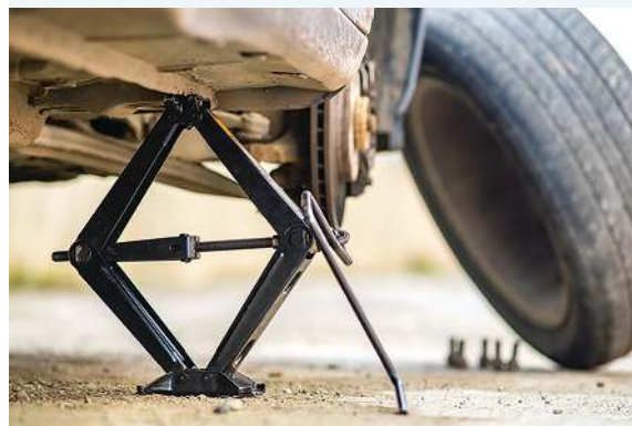
FIGURE 8.56 A car jack is a large screw that allows you to lift a heavy car with little effort. This is useful when you need to change a car tyre.
