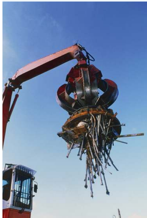
FIGURE 8.33 An electromagnet on a large crane used to lift scrap metal
