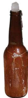
FIGURE 5.30 Oops! The reason why you shouldn't put a bottle full of water in the freezer
