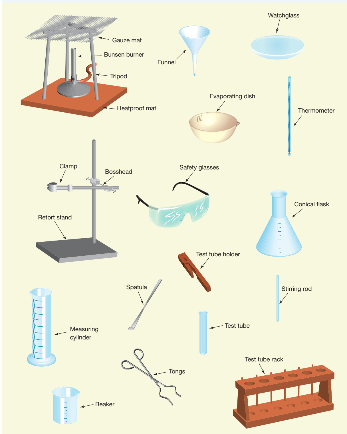
FIGURE 1.11 Some equipment that you are likely to use in the science laboratory
