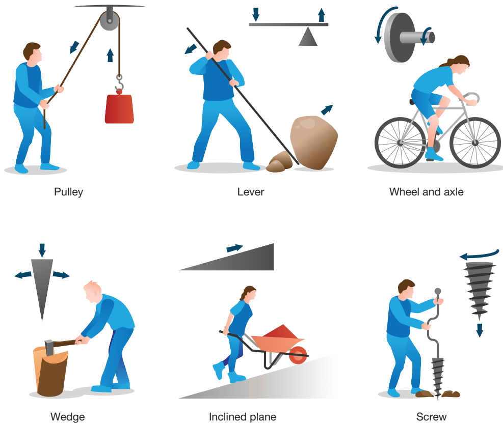
FIGURE 8.45 Some simple machines to make tasks easier
