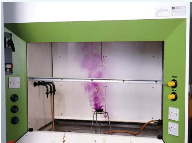
FIGURE 5.7 For safety, iodine gas is being diffused in a fume cupboard.
