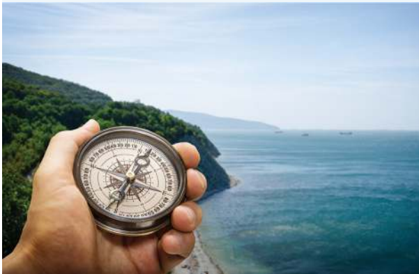
FIGURE 8.31 A compass contains a small magnetic needle that aligns with Earth's magnetic field.
