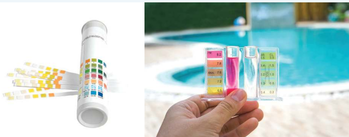
FIGURE 6.33 Pool-water test kits can be made up of test strips or a water test with an indicator showing different pH colours.
