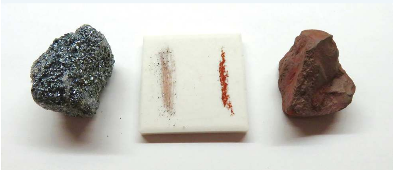
FIGURE 7.9 Streaks from minerals with a metallic lustre (left) and an earthy, dull lustre (right)
