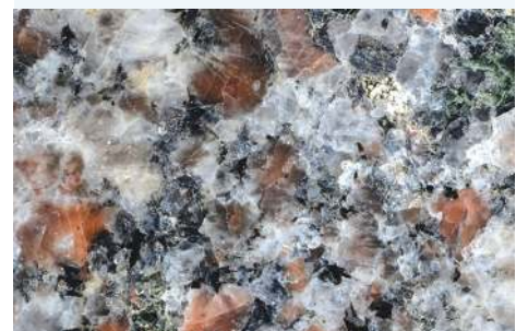
FIGURE 7.5 A close-up of granite shows how the quartz crystals grow due to overcrowding.
