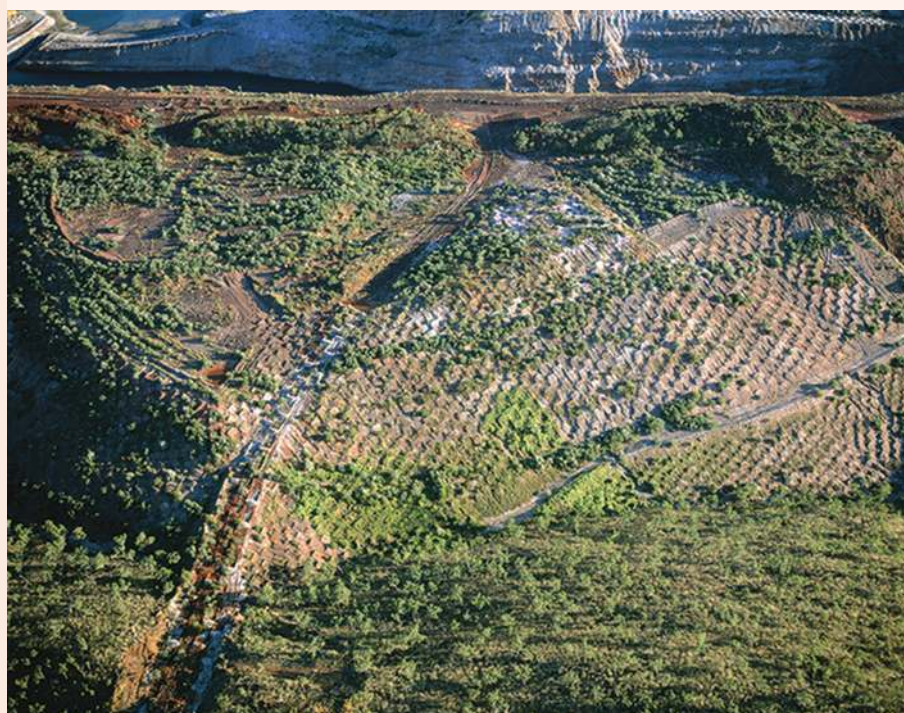
FIGURE 7.12 Resurfacing and replanting a former open-cut iron mine on Koolan Island, Western Australia
