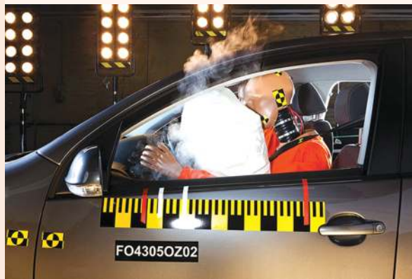
FIGURE 6.21 Airbags inflate as a result of an explosive chemical reaction.
