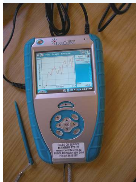
FIGURE 1.30 Some data loggers have their own touch screen and work like mini computers.
