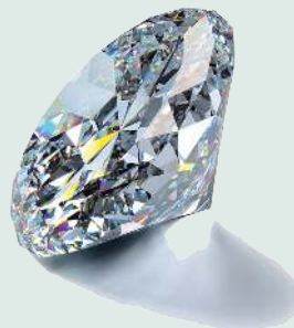
FIGURE 7.8 Faceted diamond, created by grinding a diamond on a spinning lap
