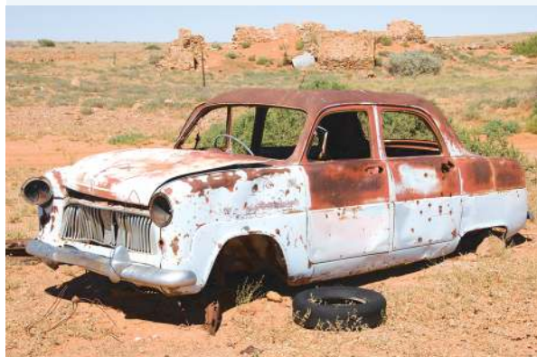
FIGURE 6.26 This wrecked car has rusted quickly because of its proximity to the sea.
