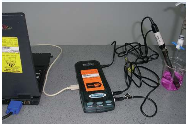
FIGURE 1.31 More basic data loggers require the use of a computer to analyse the results.
