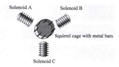
The currents in the solenoids are varied so that they create a north magnetic pole first in A, then then in B and then in C, in a clockwise rotating cycle. Which statement correctly describes what happens in the squirrel cage?
