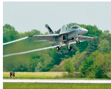
FIGURE 8.3.10 A fighter jet is successfully flight tested using a 50/50 biofuel blend. Future military and commercial jet biofuel is being researched to decrease carbon emissions.
