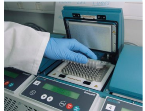
FIGURE 6.1.3 A scientist inserts a set of prepared samples into a thermocycler for PCR amplification.
