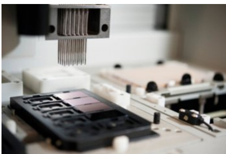
FIGURE 5.3.3 There are many technologies available to develop a SNP ‘library’ but this process can be expensive and challenging. Pictured here is a Sequenom DNA MassARRAY machine used for SNP genotyping.
