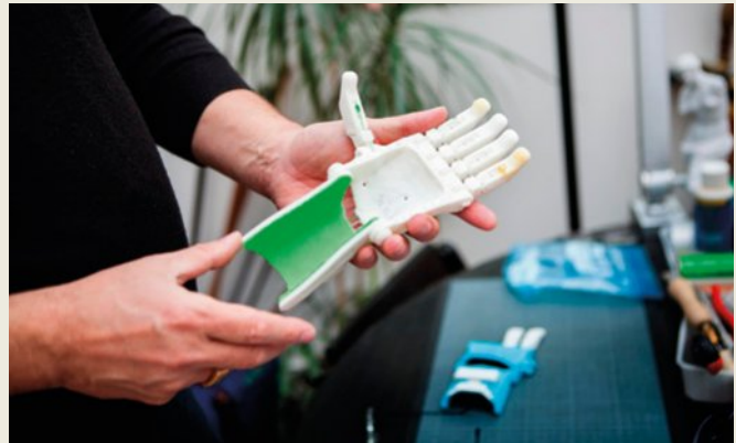
FIGURE 8.2.16 A hand prosthesis produced by a 3D medical printer promises better access to medical prosthetics.
