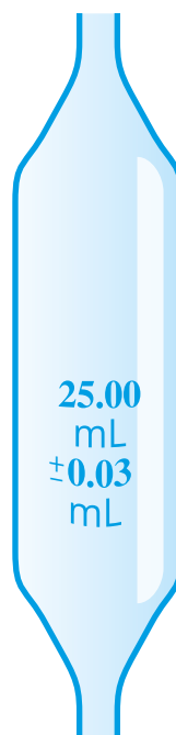
FIGURE 1.3.4 Record the uncertainty for glassware and instruments. This pipette can dispense a volume (aliquot) of 25.00 \pm 0.03 mL. When used correctly the volume dispensed will be between 24.97 mL and 25.03 mL.
