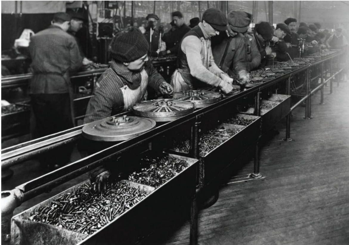
Source 6.2 History was made as the flywheel magneto, the first manufactured part to be built on a moving assembly line, passed by workers at Ford Motor Company's Highland Park plant in Michigan in the spring of 1913. Time required to assemble magnetos was reduced from 20 to five minutes. The principle was applied to all Model T assembly operations, and mass production was born.
