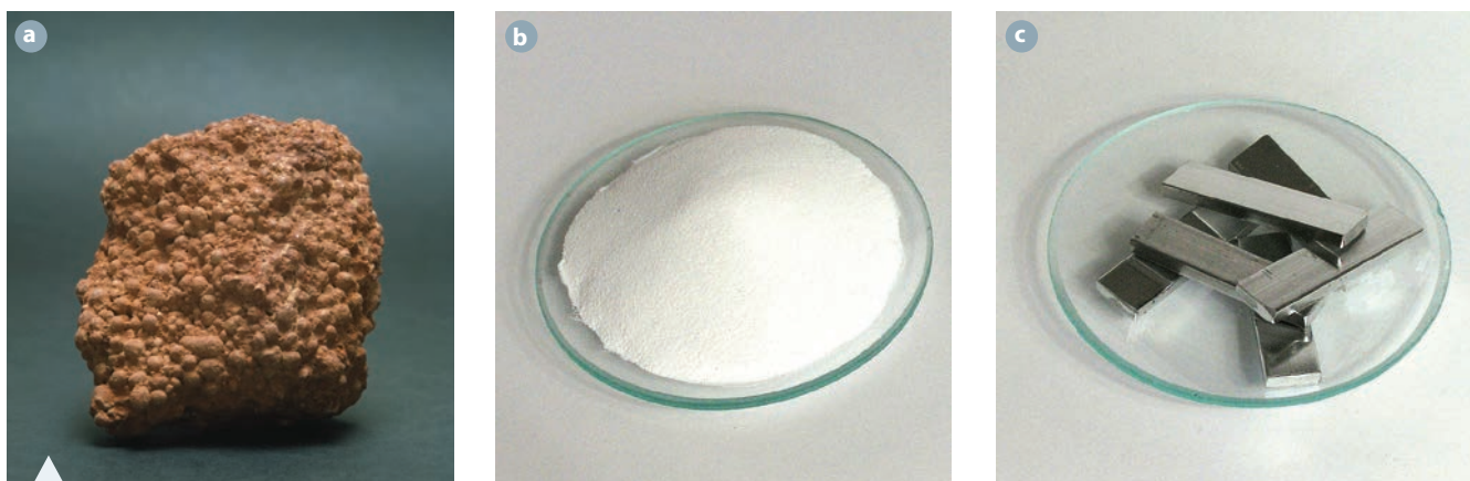
FIGURE 1.1 The substances described in Table 1.2: a bauxite, a mixture; b aluminium oxide, a compound separated from it; and c aluminium, an element obtained from the compound
