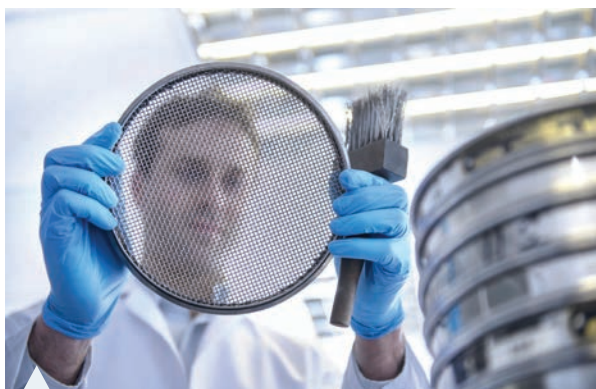
FIGURE 2.3 Industrial sieves are used to separate materials according to particle size.
