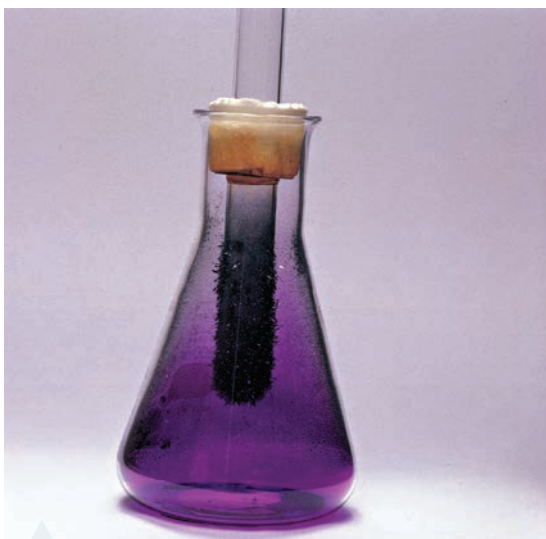
FIGURE 1.4 The sublimation and condensation of iodine solid \rightarrow gas \rightarrow solid are physical changes.
