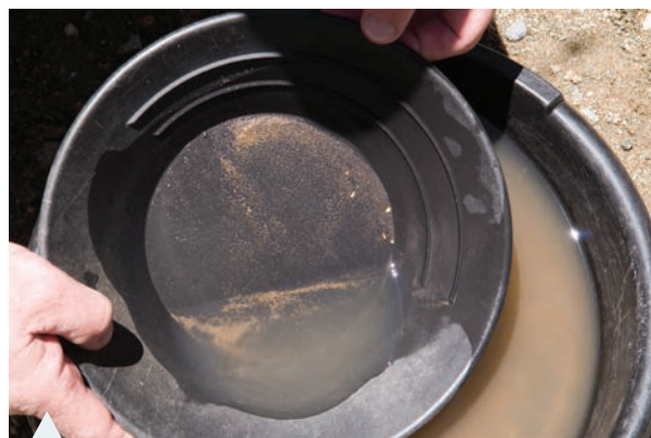
FIGURE 2.8 Panning for gold – separation based on density
