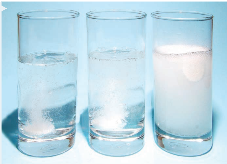
FIGURE 13.1 Tablets used to treat indigestion dissolve at different rates at different temperatures.
