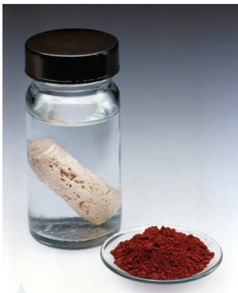
FIGURE 6.14 Two of the allotropes of phosphorus: white and red phosphorus
