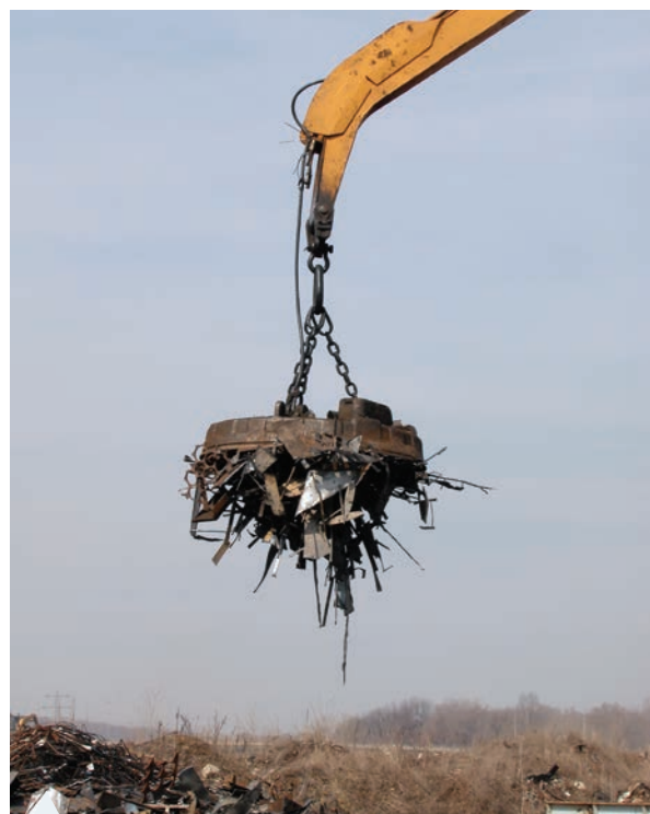
FIGURE 2.2 Magnetism is widely used to sort ferrous (magnetic) metals from other metals.
