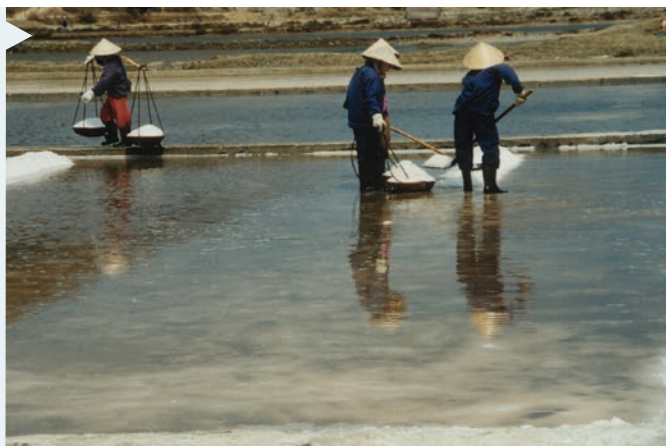
FIGURE 2.1 Salt can be separated from sea water using evaporation. In Vietnam this is done manually, as shown, while in Australia machines are generally used.
