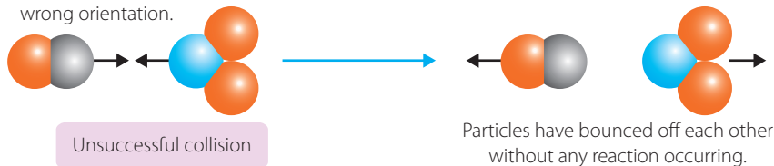
FIGURE 13.8 Correct particle orientation is required for reaction to occur.
