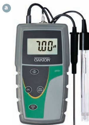
FIGURE 1.7 a A typical small pH meter; b a page from the user manual giving the precision on various scales
