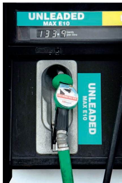
FIGURE 9.1 Ethanol, with an alcohol functional group, is used as an additive in petrol.
