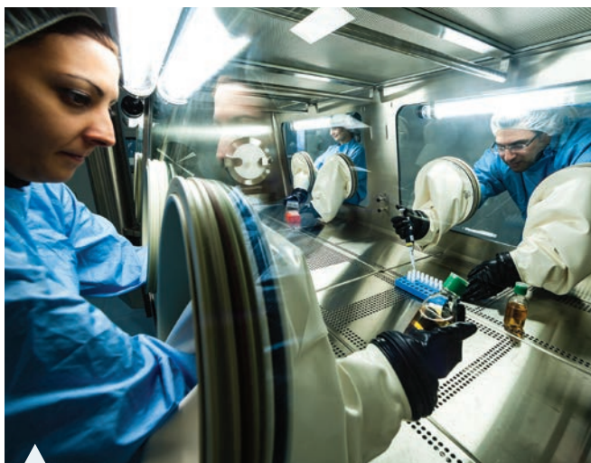
FIGURE 10.3 A chemist working in a containment system to isolate the chemical vapours
