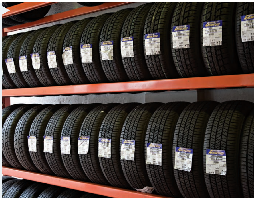
FIGURE 13.11 Car tyres are made from a mixture of natural rubber and synthetic rubber – a styrene– butadiene copolymer.
