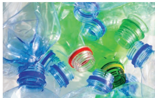
FIGURE 13.2 Plastic drink bottles are made of a thermoplastic polymer so can be easily recycled.
