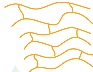
FIGURE 13.13 Cross-linking joins chains to each other.
