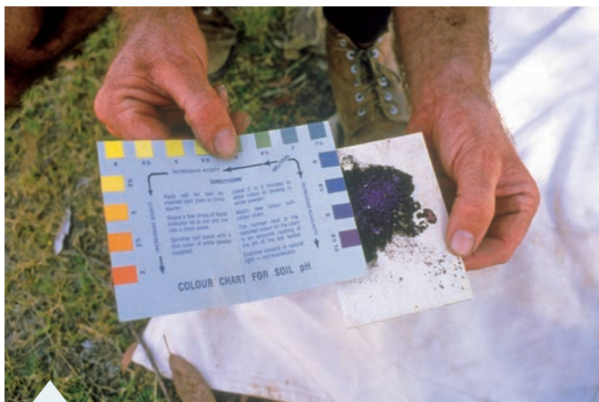
FIGURE 6.6 Checking the approximate pH of soil using an indicator colour chart
