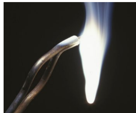
FIGURE 12.1.3 Magnesium ribbon burns brightly when heated in air to form a white powder, magnesium oxide.
