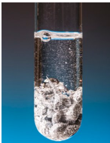
FIGURE 10.6.1 Hydrogen gas is produced from the reaction of zinc with dilute hydrochloric acid.
