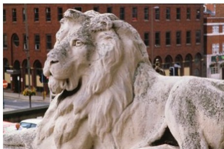
FIGURE 13.3.3 This limestone statue has become pitted in recent years. Limestone (calcium carbonate) reacts more rapidly with the increased acid concentration in rainwater.
