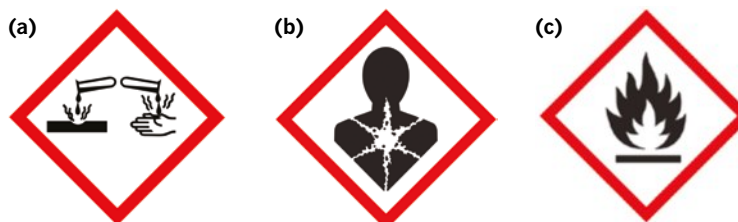
FIGURE 1.2.8 On 1 January 2017, the GHS (Globally Harmonized System of Classification and Labelling of Chemicals) pictograms were introduced in Australia. These are used for labelling chemical containers and in safety data sheets. Some of the pictograms you may see denote chemicals that (a) are corrosive, (b) pose a health hazard or (c) are flammable.
