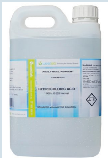
Figure 8.4.7 An alternative to preparing standard solutions is to purchase them from certified laboratories.
