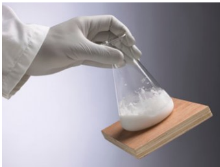
FIGURE 16.2.2 Solid barium hydroxide and solid ammonium chloride have been mixed in a flask that is sitting on a damp piece of wood. Although the reaction is endothermic (its temperature drops to well below 0°C and freezes the flask to the wood), it occurs spontaneously due to an increase in entropy of the system.
