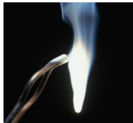
FIGURE 10.1.5 Magnesium ribbon and the oxygen in the air are reactants. The white powder forming on the tongs is the product, magnesium oxide.
