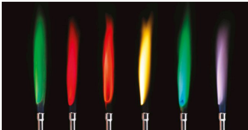
FIGURE 3.4.3 The colour of each flame is caused by the different metal compounds present and can be used to identify the metals. The flame colours shown here are due to (from left to right): barium (yellow-green), lithium (crimson), strontium (scarlet), sodium (yellow), copper (green) and potassium (lilac).
