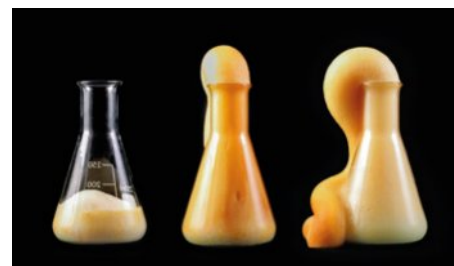
FIGURE 10.3.1 The elephant’s toothpaste decomposition reaction begins with a hydrogen peroxide sample. A catalyst causes rapid decomposition, producing what is called ‘elephant’s toothpaste’.
