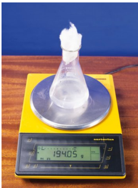
FIGURE 13.2.3 Apparatus to monitor the mass of carbon dioxide gas released during a reaction between marble chips and an acid.
