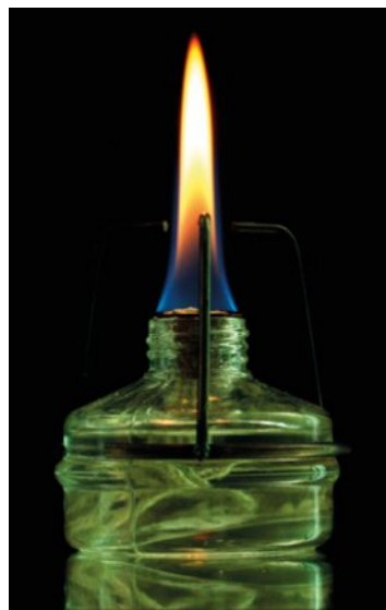
FIGURE 10.4.4 Alcohol burners or spirit lamps are used in some science laboratories. They burn liquid alcohols, such as ethanol, and produce carbon dioxide and water. Spirit lamps produce a smaller, cooler flame than Bunsen burners.
