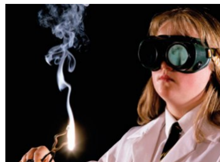
FIGURE 11.1.5 Magnesium ribbon burns brightly when heated in air to form a white powder, magnesium oxide.
