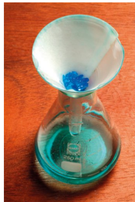
FIGURE 2.3.4 When water is evaporated from a solution of copper(II) sulfate, crystals of copper(II) sulfate precipitate out. The crystals can then be filtered to separate them from the remaining solution. The filtrate remains blue, which means that not all of the copper(II) sulfate has precipitated.
