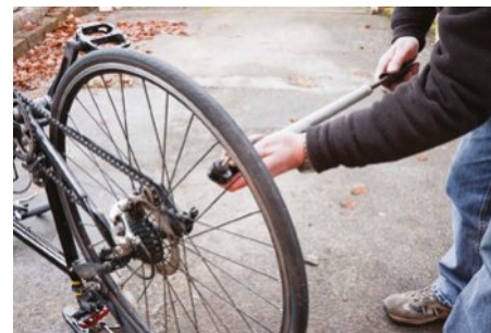
FIGURE 9.1.3 Pumping more air into a tyre increases the pressure in the tyre because more particles are being pumped into a nearly fixed volume.
