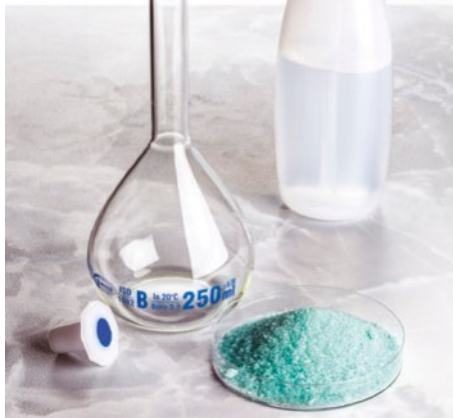
FIGURE 8.4.1 Apparatus and materials needed to prepare a standard solution. The measured mass of solid will be dissolved in water in a volumetric flask to make an accurate volume of solution.
