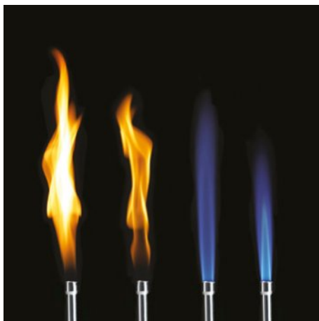
FIGURE 10.4.2 The yellow flame of a Bunsen burner is due to incomplete combustion and produces carbon. The blue flame is the hotter flame that occurs when the collar hole is open and more oxygen is allowed into the reaction.
