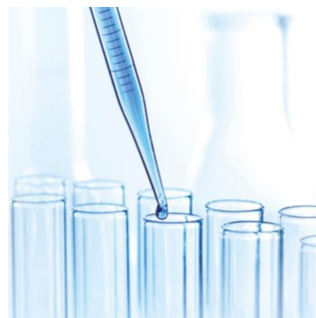
FIGURE 1.2.3 A 5 mL graduated pipette can measure volumes to an accuracy of one-hundredth of a millilitre, or 5.00 \pm 0.01 mL. The pipette has major divisions of 1 mL and minor divisions of 0.1 mL. You can estimate to 0.01 mL and record volumes to two decimal places, for example: 3.80 mL or 4.52 mL.
