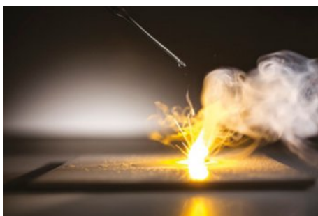
FIGURE 12.4.1 Water dropped onto sodium metal. Sodium is highly reactive; the products are sodium hydroxide and hydrogen gas.
