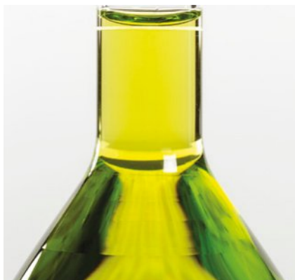
FIGURE 8.4.4 This close-up view of the neck of a standard flask shows that the bottom of the meniscus is level with the white graduation line.
