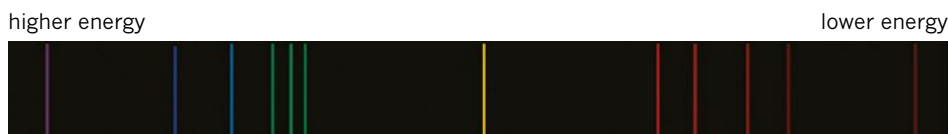
FIGURE 3.4.6 The emission spectrum of helium is made up of lines ranging from violet to red in colour.
