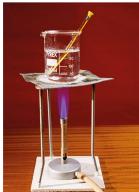
FIGURE 15.1.1 Heating water in a beaker over a Bunsen burner. Pure water boils at a temperature of 100°C at an atmospheric pressure of 101.3 kPa.
