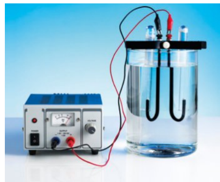
FIGURE 10.3.6 Electrical energy from a power supply is causing water to decompose to hydrogen gas at one electrode and oxygen gas at the other. The gases can be collected by placing a container over the electrodes.
