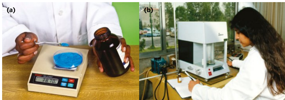
FIGURE 8.4.2 (a) A top-loading balance and (b) an analytical balance can be used to accurately weigh substances used in chemical analysis.
