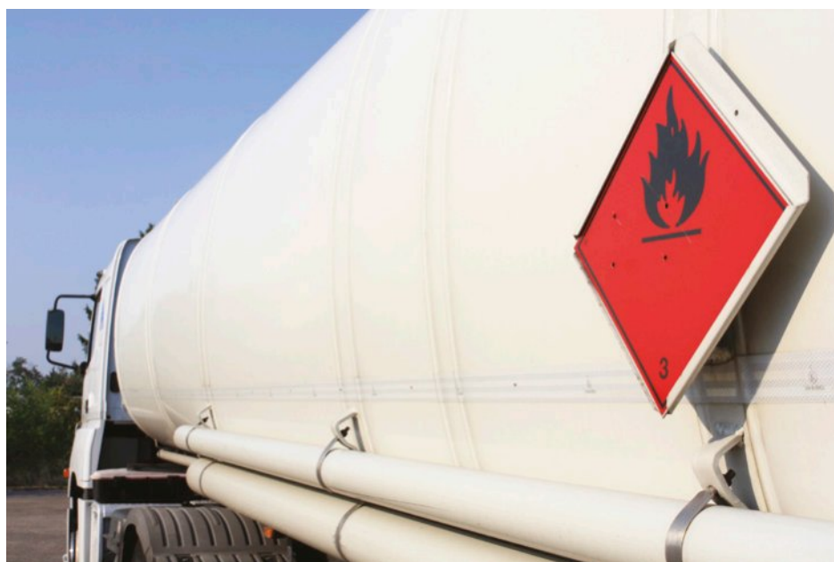
FIGURE 1.2.7 Trucks transporting hazardous substances such as flammable liquids have hazard symbols attached.
