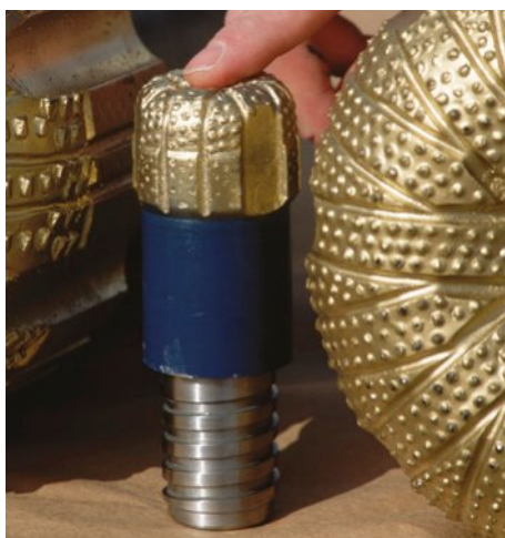
FIGURE 5.5.2 Diamond-tipped drills, which are used to drill through rock, mining for oil and natural gas.
