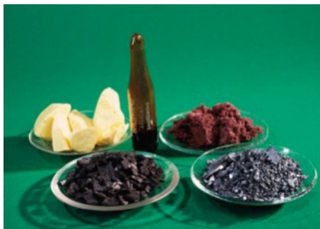
FIGURE 2.5.2 Non-metals have very different physical appearances, for example, yellow sulfur, brown bromine in a flask, red phosphorus, dull grey iodine and solid black carbon.
