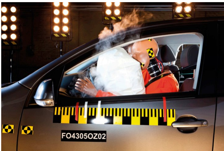
FIGURE 10.3.4 A collision triggers the release of heat energy. This heat energy leads to the decomposition of sodium azide and the formation of nitrogen gas, which inflates the airbag.
