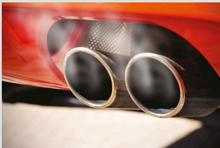
FIGURE 10.4.3 Car exhaust gases can contain high levels of carbon monoxide as a result of incomplete combustion of fuels.
