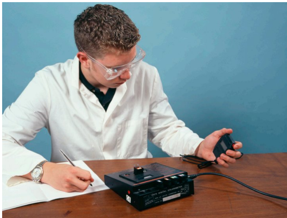
FIGURE 13.2.7 A student using a colorimeter to monitor the rate of reaction between potassium permanganate and oxalic acid: 2\text{MnO}_4^-(\text{aq}) + 5\text{H}_2\text{C}_2\text{O}_4(\text{aq}) + 6\text{H}^+(\text{aq}) \rightarrow 2\text{Mn}^{2+}(\text{aq}) + 10\text{CO}_2(\text{g}) + 8\text{H}_2\text{O}(\text{l})
