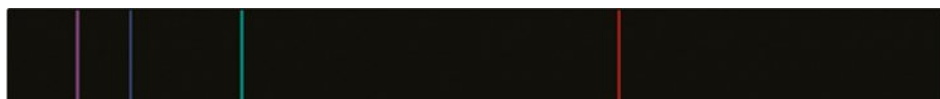
FIGURE 3.4.10 The emission spectrum of the hydrogen atom has four lines in the visible range: violet, blue, green and red.
