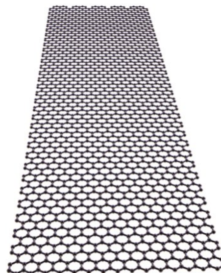
FIGURE 5.5.10 Graphene is a single layer sheet with the same arrangement as the layers stacked in graphite.
