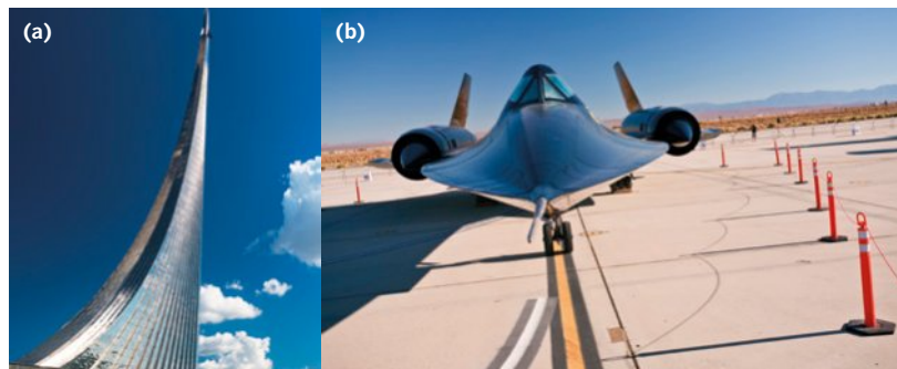
FIGURE 5.1.1 The metal titanium has many uses, including in (a) the spectacular curved space museum building in Moscow and (b) the SR-71 Blackbird reconnaissance aircraft.
