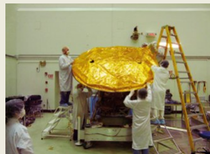
FIGURE 11.1.7 A gold-coated radiation shield is installed on a section of a satellite.
