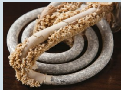
FIGURE 10.5.6 The accumulation of limescale on domestic kettle elements is the result of the precipitation of calcium carbonate when water is repeatedly boiled.
