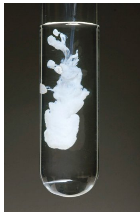
FIGURE 10.5.3 Mixing aqueous solutions of sodium chloride and silver nitrate produces a solid, which is an example of a precipitate.
