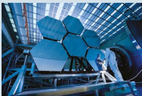
FIGURE 5.1.7 These are some of the 18 mirror segments of the James Webb Space Telescope. The mirrors are supported by beryllium ribs that will maintain the mirror's shape under extreme conditions.
