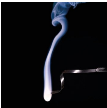
FIGURE 2.5.6 A ribbon of magnesium burning in air. When heated in air, it burns with a bright, white flame.
