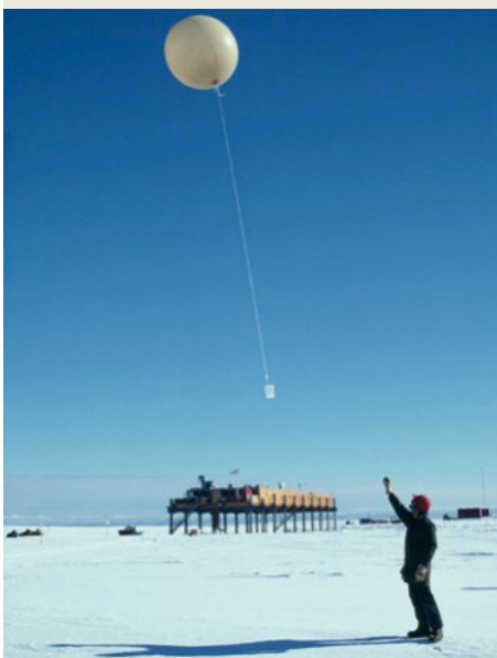
FIGURE 9.2.3 A researcher launching a radiosonde weather balloon, which is carrying a package of instruments. Study of the atmosphere allows more accurate weather forecasting and enables environmental change to be monitored. Photographed at the Halley Research Station, Antarctica.
