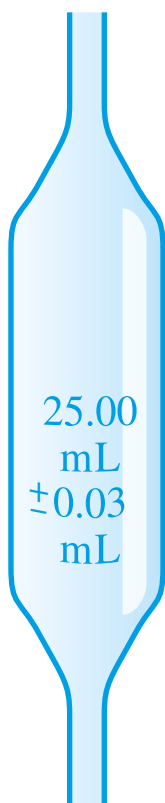
FIGURE 1.3.3 Record the uncertainty for glassware and instruments. This pipette can dispense a volume (aliquot) of 25.00 \pm 0.03 \text{ mL} . When it is used correctly, the volume dispensed will be between 24.97 \text{ mL} and 25.03 \text{ mL} .
