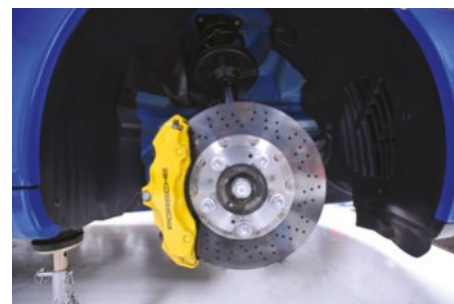
FIGURE 5.2.4 Ceramic brake discs work more effectively than steel ones at high temperatures. A ceramic brake disc contains ionic compounds that have very high melting temperatures and are better than metals at withstanding the heat produced by braking.
