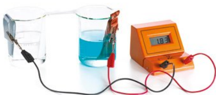
FIGURE 12.3.2 Construction of a galvanic cell from simple laboratory equipment.
