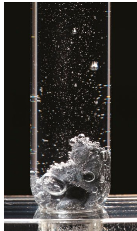
FIGURE 14.2.4 When zinc comes into contact with hydrochloric acid, it reacts almost immediately. The reactants have sufficient energy to overcome the activation energy barrier.
