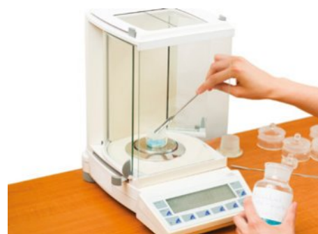
FIGURE 7.2.1 A digital balance is a simple piece of laboratory equipment used for weighing.
