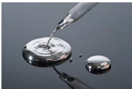
FIGURE 4.2.2 Mercury is different to the rest of the d -block elements because it is liquid at room temperature ( 25^{\circ}\text{C} ), whereas the rest of the d -block elements are solid at room temperature.
