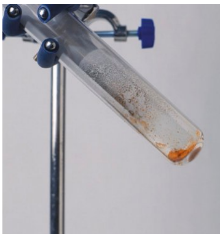
FIGURE 2.1.5 The red powder in this test-tube is mercuric oxide. If you look closely at the test-tube, you will see beads of liquid mercury forming from the decomposition of the compound.
