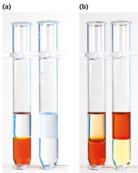
FIGURE 11.1.8 (a) When an alkene is added to aqueous bromine, the alkene reacts with the coloured bromine and the solution loses colour. (b) When an alkane is added to aqueous bromine, no addition reaction occurs, so the colour does not change.
