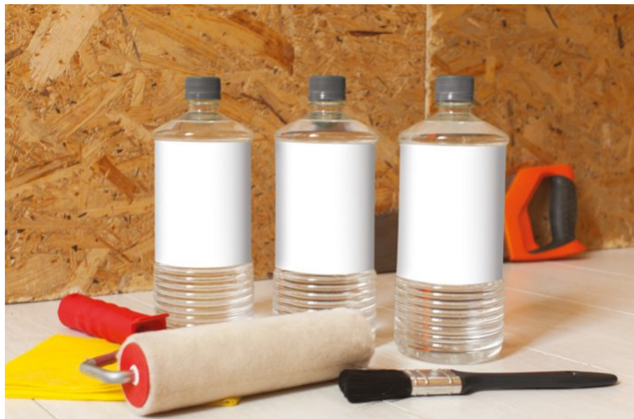
FIGURE 10.1.8 White spirit contains a mixture of alkanes. It is a useful solvent for other non-polar liquids.
