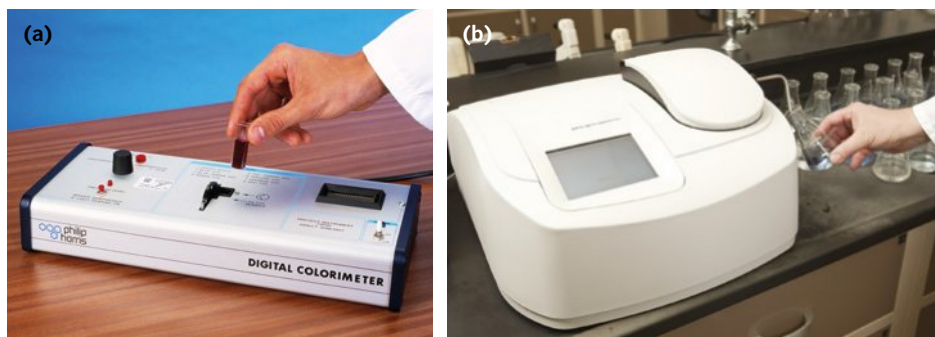
FIGURE 15.4.12 (a) A portable colorimeter. A solution sample is inserted into this unit in a small plastic cell. (b) A laboratory UV–visible spectrometer.
