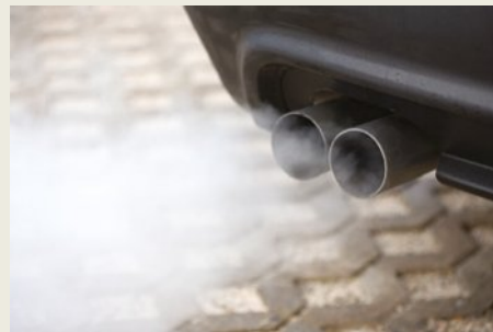
FIGURE 4.1.5 Carbon monoxide gas is formed when a hydrocarbon fuel such as petrol is burnt in a limited supply of oxygen.
