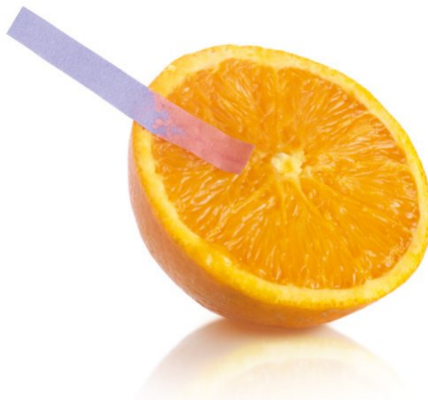
FIGURE 7.2.5 Blue litmus paper turns red when exposed to the citric acid in an orange.
