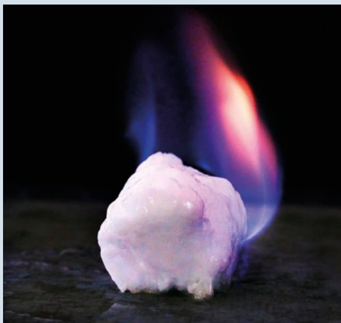
FIGURE 11.1.2 The combustion of methane hydrate looks like burning ice. As the solid melts, methane gas is released, providing the fuel for the combustion reaction.
