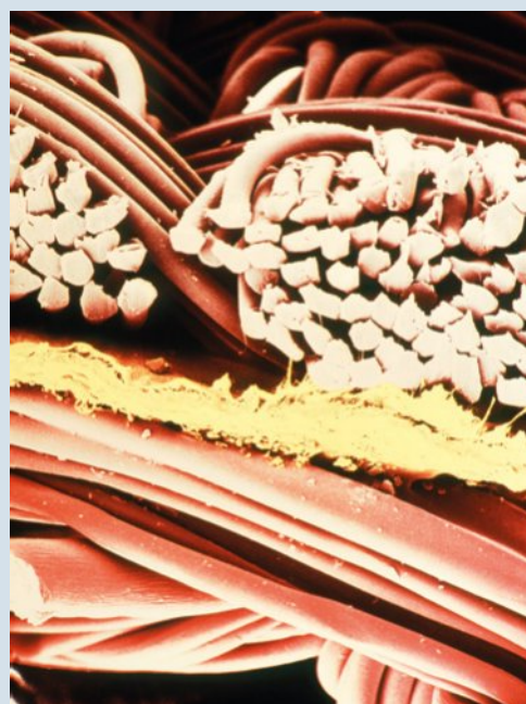
FIGURE 14.1.22 Scanning electron micrograph of Gore-Tex fabric. The yellow layer is Teflon. The spaces in this layer are small enough to prevent water passing through but large enough to allow water vapour to pass through.
