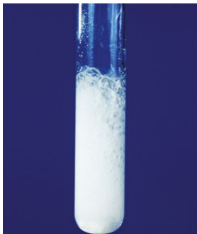
FIGURE 16.1.5 There is vigorous effervescence when solid sodium hydrogen carbonate is added to a carboxylic acid.
