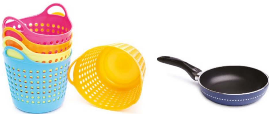
FIGURE 14.1.3 A plastic basket has plastic properties, whereas a polymer frying pan handle does not.
