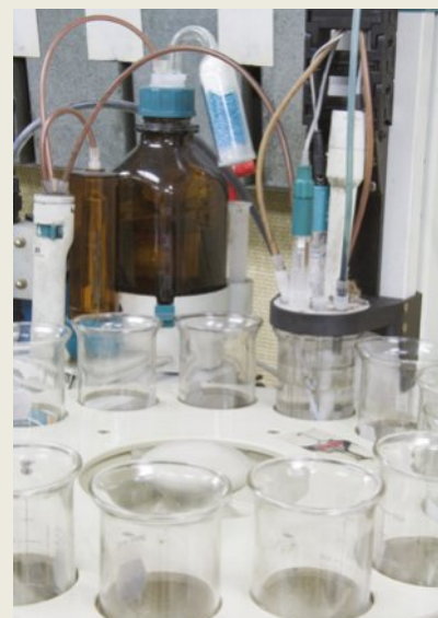
FIGURE 8.2.7 Automated titrators can rapidly analyse a large number of samples.
