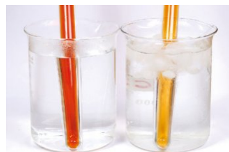
FIGURE 4.2.7 Equilibrium mixtures of \text{NO}_2 and \text{N}_2\text{O}_4 in baths of hot water (left) and ice water (right). Heating the mixture favours the formation of brown \text{NO}_2 gas.
