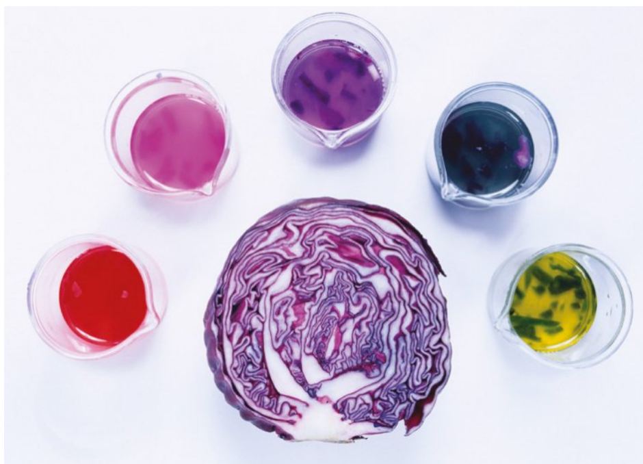
FIGURE 6.1.4 Natural acid–base indicators are found in plants such as red cabbage. Red cabbage extract turns a different colour in (from left to right) concentrated acid, dilute acid, neutral solution, dilute base and concentrated base.
