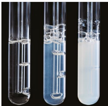
FIGURE 16.1.6 When carbon dioxide is bubbled through limewater, the limewater turns cloudy.
