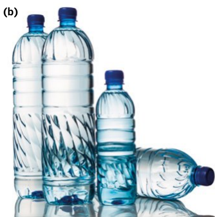
FIGURE 14.2.2 Polyethene terephthalate (PET) is formed when benzene-1,4-dioic acid reacts with ethane-1,2-diol. The PET is linked by ester groups, which is why it is part of the polyester family of polymers.
