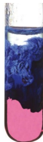
FIGURE 15.2.5 A royal blue precipitate will form when SO 4 2- ions are added to a solution containing Co 2+ ions.
