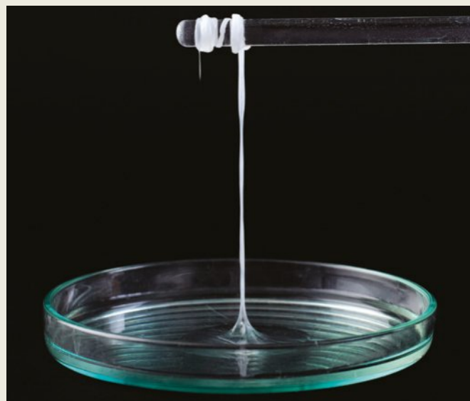
FIGURE 14.2.9 Nylon forms at the interface between the two monomers.
