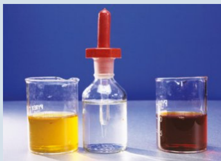
FIGURE 3.1.2 Making fake blood. An \text{Fe}^{3+} solution (left) is mixed with an \text{SCN}^- solution (centre) to produce a blood-red equilibrium mixture of \text{Fe}^{3+} , \text{SCN}^- and \text{FeSCN}^{2+} (right).
