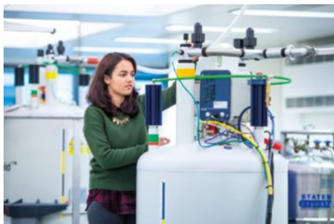
FIGURE 16.3.1 A research chemist places a sample tube into an NMR spectrometer.
