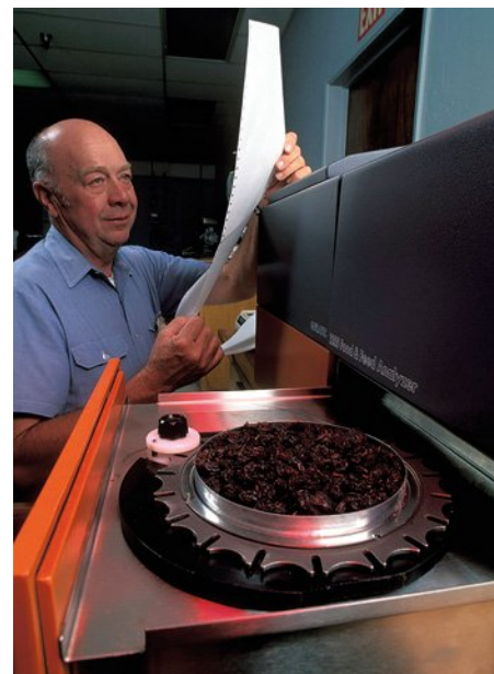
FIGURE 16.2.3 A food chemist uses an infrared spectrometer to evaluate the quality of raisins.
