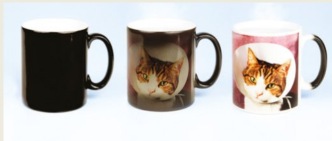
FIGURE 3.2.2 The coating on this cup is temperature-sensitive, revealing the picture below it when hot water is added to the cup.
