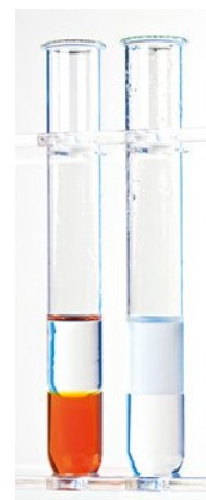
FIGURE 16.1.2 Bromine changes colour when it reacts with an alkene.
