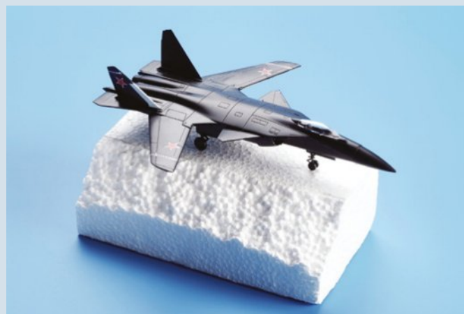
FIGURE 14.1.20 The model plane is made from rigid polystyrene, while the white base is expanded polystyrene foam.
