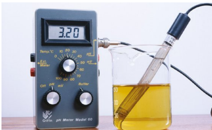
FIGURE 7.2.2 A pH meter is used to measure the acidity of a solution.
