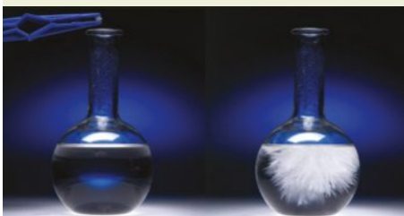
FIGURE 5.2.6 Crystals of sodium acetate form after a seed crystal is added to a supersaturated solution of the compound.
