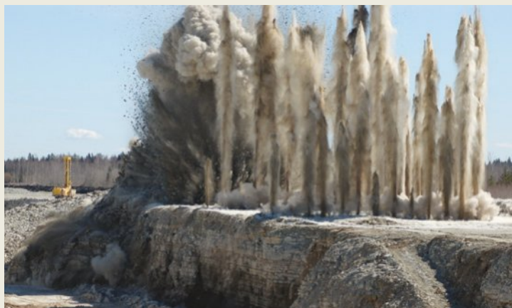
FIGURE 2.2.12 Controlled blasting in an open-cut mine. The explosive reaction is a non-equilibrium system.
