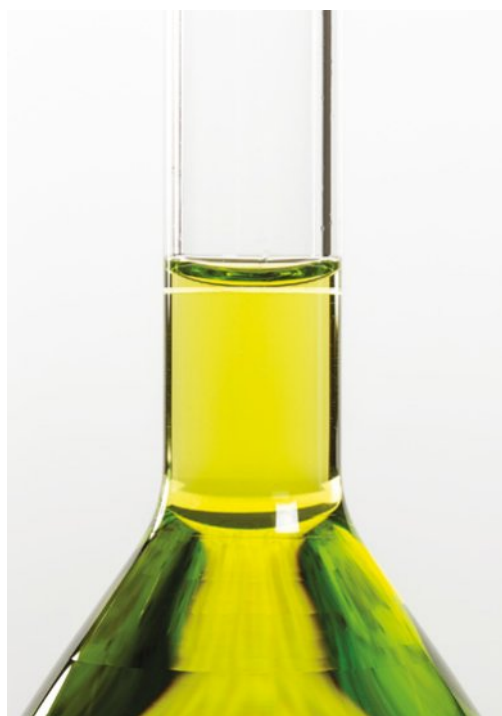
FIGURE 8.23 This close-up view of the neck of a standard flask shows the bottom of the meniscus is level with the white graduation (measuring scale) line.
