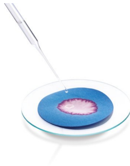
FIGURE 2.1.7 Blue dehydrated cobalt(II) chloride paper turns pink in the presence of water.
