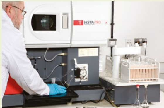
FIGURE 15.5.11 An inductively coupled plasma (ICP) analyser.
