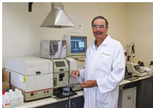
FIGURE 15.5.10 An analytical chemist uses AAS to determine the concentration of metals in food samples.
