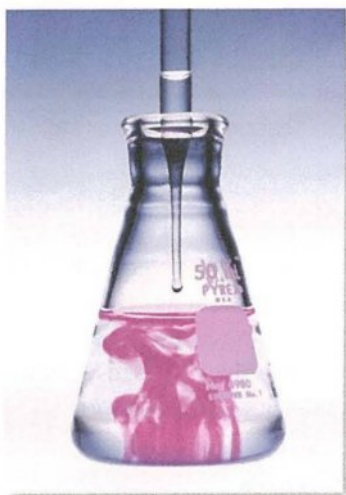
Figure 38.6 A base being added to an acid in a flask with a few drops of phenolphthalein present. The colour is changing from colourless to red.
