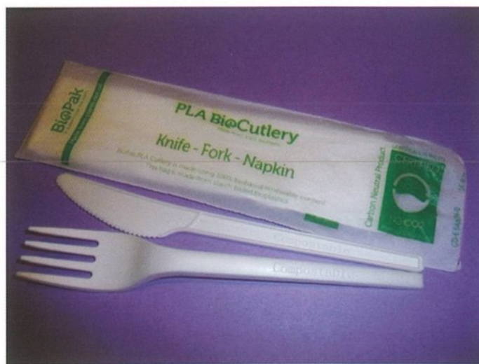
Figure 58.6 Cutlery made from biobased renewable substances. The bag is made from a starch based polymer.
