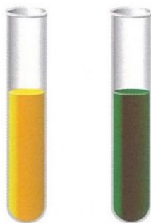
Figure 31.1 Reduction of dichromate to chromate ions.
