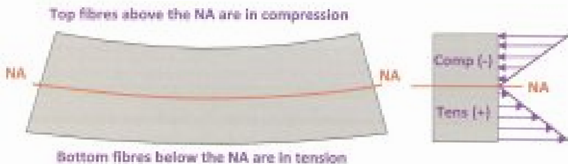
Figure 2.6: Beam undergoing bending whereby top is in compression and bottom in tension. NA in the middle.
