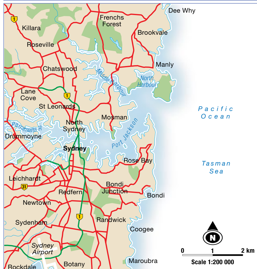
Figure 1.2c Different scales can show different levels of detail. The top map is drawn at a scale of 1:400 000 and the bottom map at 1:200 000.
