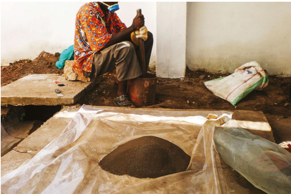
Source 19.18 Coltan ore being ground
