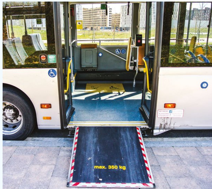
Source 7.17 A bus with ramp access for those with a mobility disability, such as a wheelchair
