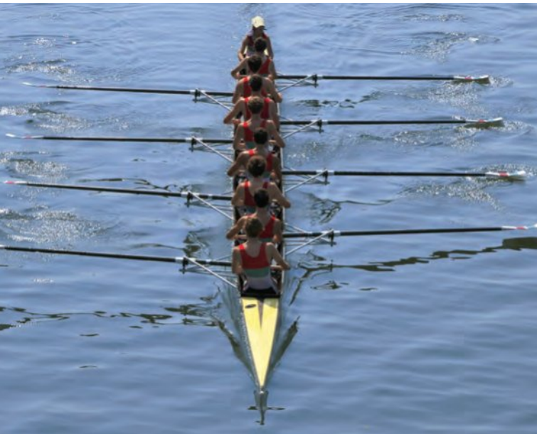
Figure 2.73 Row boats are made as narrow as possible to minimise profile drag
