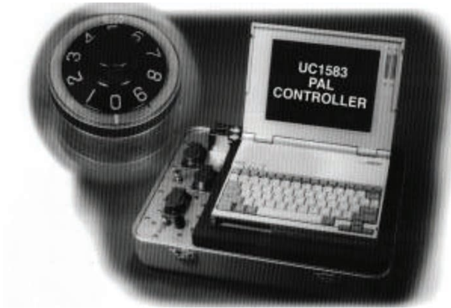
SOURCE 10.58 A Permissive Action Link (PAL) is a security device for a nuclear weapon designed to prevent unauthorised arming or detonation.
