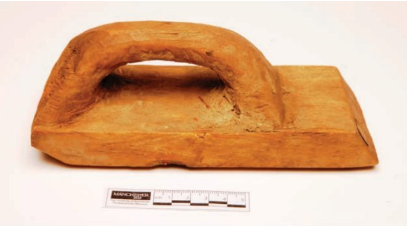
FIGURE 2.26 A plasterer's float
