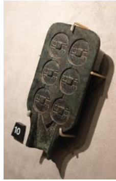
FIGURE 7.24 A mould for making ban liang coins
