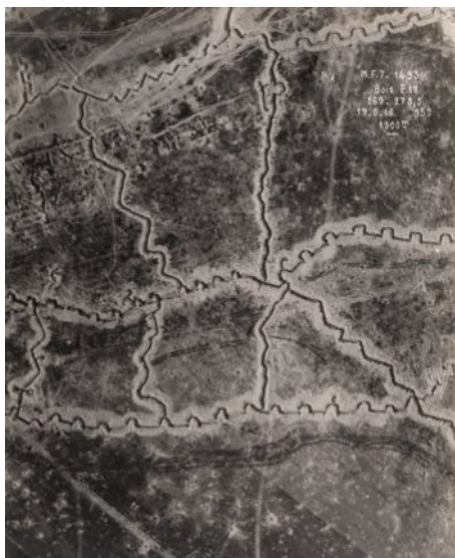
Figure 8.3 An aerial view of a section of the Western Front. Notice the tessellated (shaped like teeth) pattern of the trenches.
