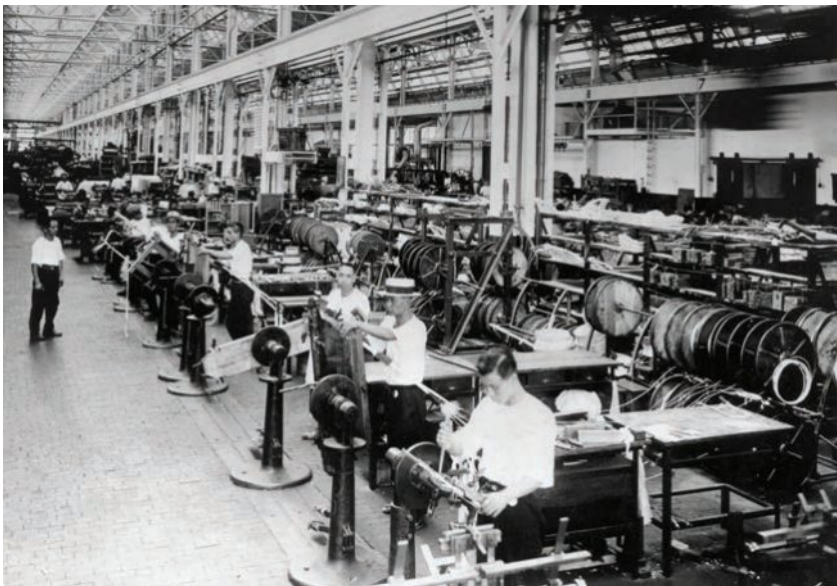
Figure 3.11 Workers winding induction regulator coils in a Shibaura Engineering Works plant, 1927
