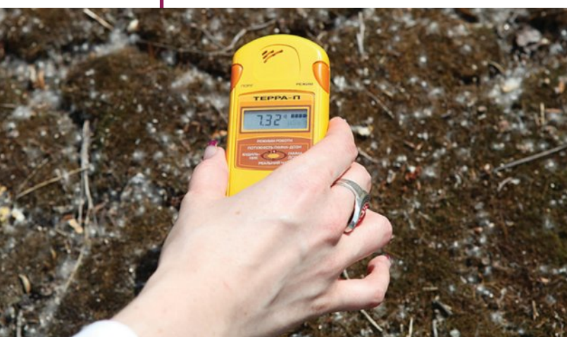
Figure 11.5 Reading the radiation levels with a Geiger counter in front of the reactor in Chernobyl, Ukraine.
