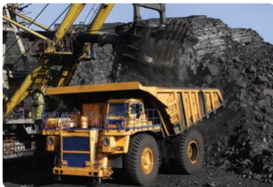
A typical large mining truck has a capacity of 140 tonnes.
