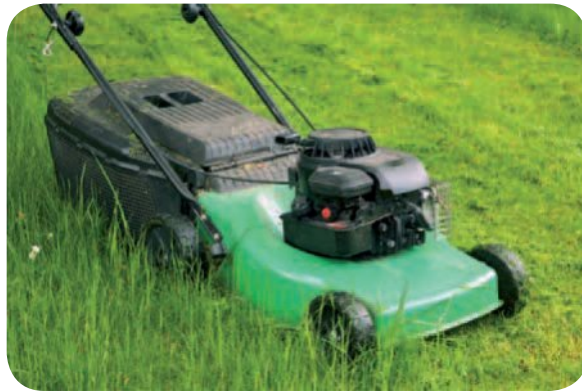
Two-stroke lawnmowers run on petrol and oil mixed in a certain ratio.
