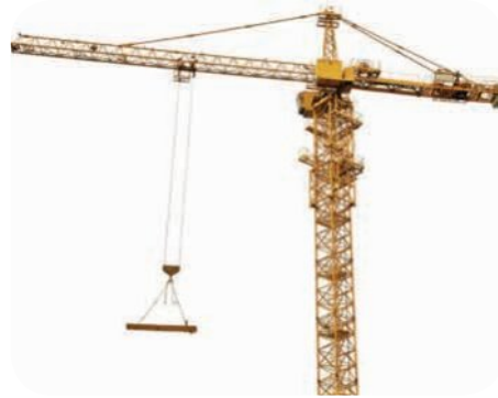
Engineers have used many triangles in the design of cranes to make them strong and rigid but relatively lightweight.
