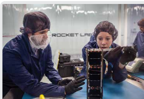
CubeSats, designed by space engineers for scientific research, are miniaturised satellites made of one or more cubes with 10 cm sides. Their surface area is used for solar power panels.
