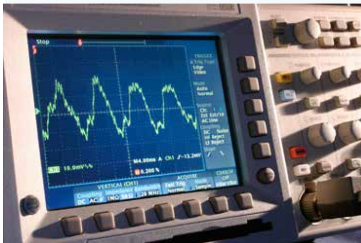
FIGURE 9.34 The waveform shown is produced by plucking the A string of a guitar. The pattern on the CRO screen results from the superposition of waves with frequencies corresponding to the fundamental and subsequent harmonics.
