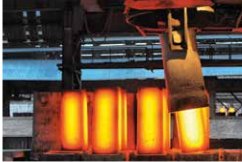
FIGURE 11.3 This steel is nearly 1000 °C and has recently been poured in a mould to shape it. The steel will continue to glow until it has cooled to about 400 °C.
