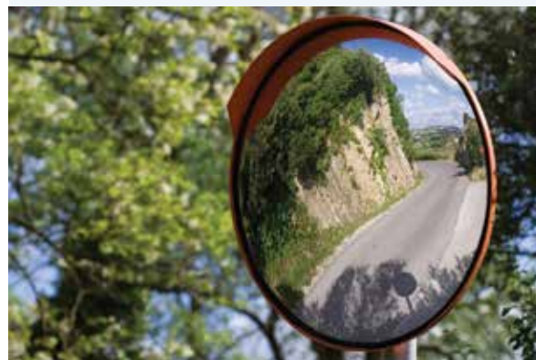
FIGURE 10.38 Convex mirrors are often used to help improve vision around corners.
