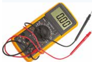
FIGURE 13.13 A digital multimeter, which can measure current, voltage drop and resistance.
