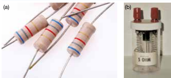
FIGURE 13.26 Examples of (a) carbon resistors and (b) a coiled wire resistor.
