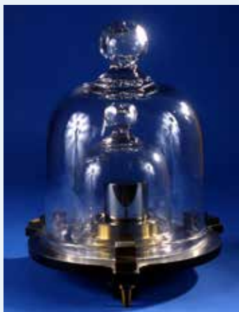
FIGURE 1.4 The National prototype kilogram K20 is one of two prototypes stored at the US National Institute of Standards and Technology in Gaithersburg, Maryland. Many countries have their own copies of the international prototype. This image is a replica for public display, shown as it is normally stored, under two bell jars. It is approximately 39.17 mm in diameter and height.
