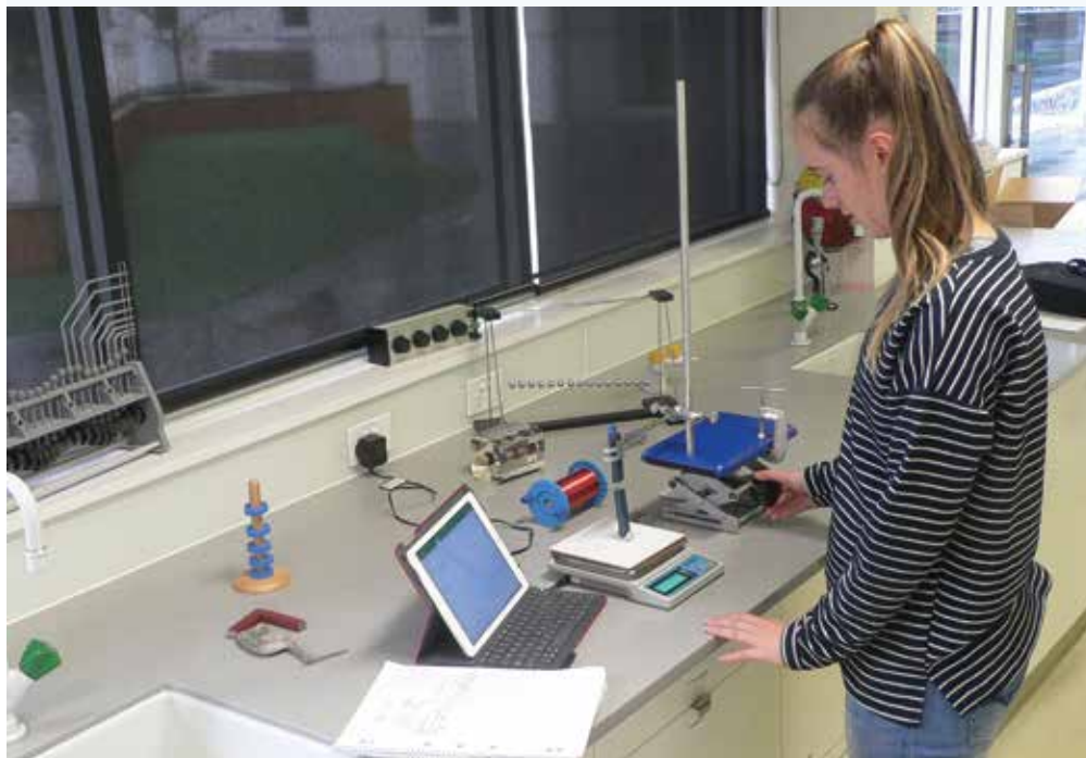
FIGURE 1.1 This student is investigating the relationship between the strength of attraction between two bar magnets and the distance separating them.
