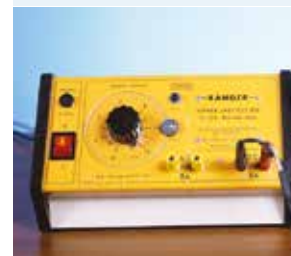
FIGURE 13.15 A power pack is used in school laboratories to supply electrical potential energy to a circuit.
