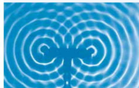
FIGURE 8.12 An interference pattern obtained in water by using two point sources that are in phase.
