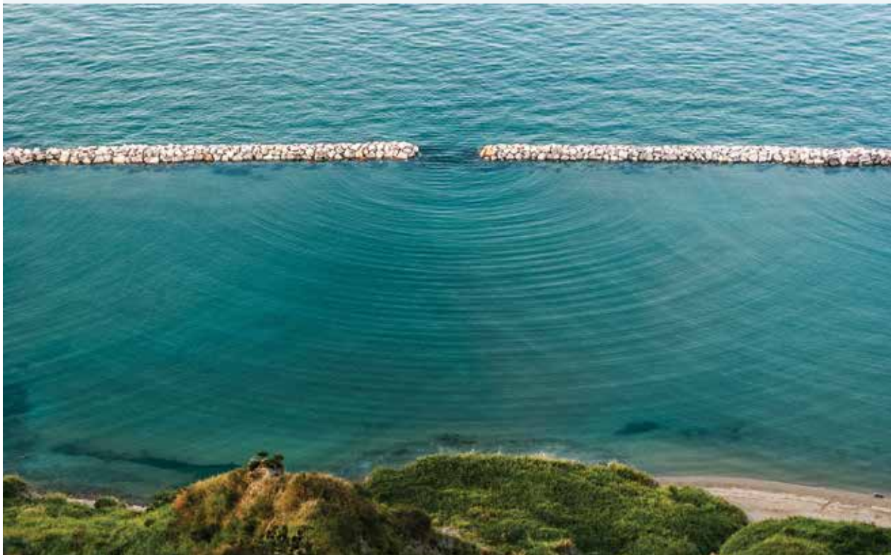
FIGURE 8.1 Ocean waves entering a gap in a barrier will experience diffraction — a behaviour exhibited by all waves under the right circumstances.
