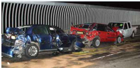
FIGURE 6.8 Crumple zones at the front and rear of cars reduce the rate of change of momentum of the car and its occupants during a collision.
