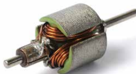
FIGURE 14.43 Commutator and coil from a hair dryer.
