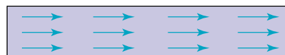
(c) All domains face the same direction, resulting in a strong magnet.
