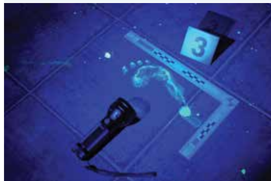
FIGURE 10.4 When liquid Luminol comes into contact with the iron in blood haemoglobin in the presence of ultraviolet light, the blood is luminous as a result of the chemical reaction rather than because of incandescence.
