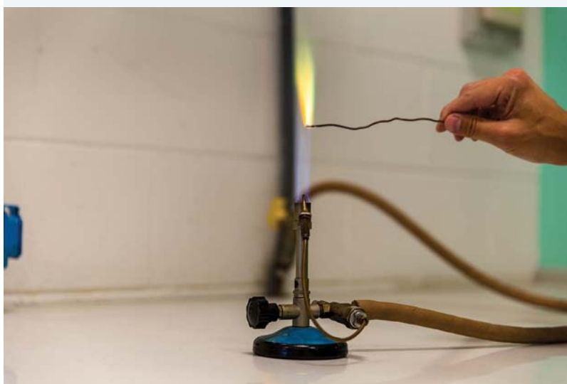
FIGURE 8.20 Burning elements in a flame is called a flame test. Different elements can produce different and vivid colours when burned in a flame.
