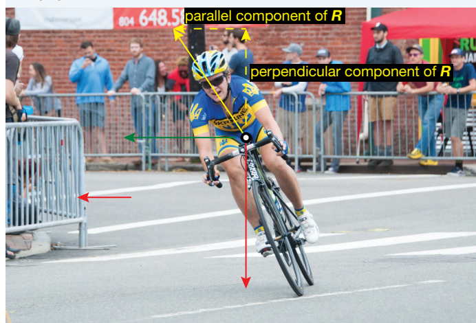
FIGURE 2.19 Leaning into a corner increases the size of the net force, allowing a higher speed while cornering. The sideways friction is greater, and the reaction force of the ground has a component towards the centre of the circular motion.
