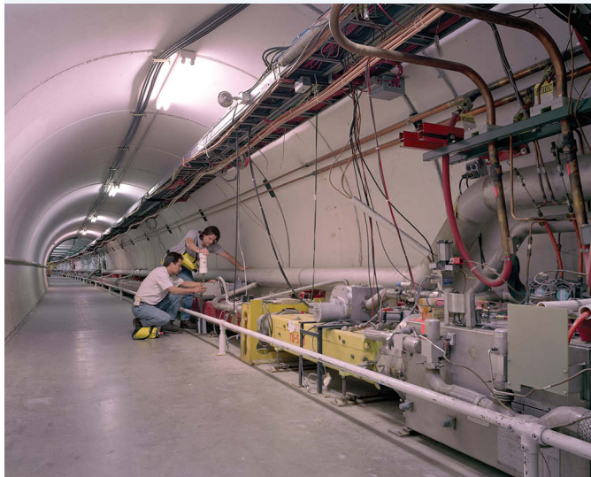
FIGURE 16.13 Part of the 6.28 km (circumference) Fermilab Tevatron accelerator. The yellow and red sections on the floor are parts of the new accelerator, which can accelerate protons to nearly 1000 GeV.
