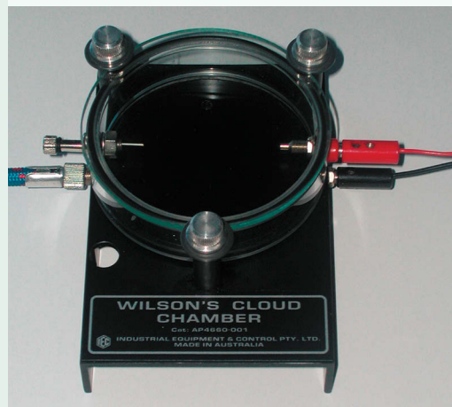
FIGURE 16.16 A Wilson cloud chamber.
