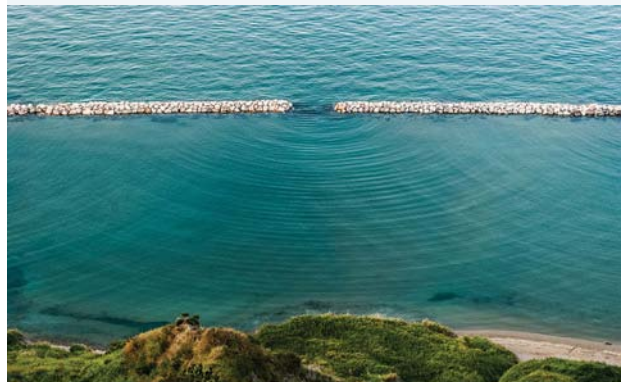
FIGURE 9.3 This aerial photograph shows water waves passing through a gap in a breakwater. The waves that have already passed through can be seen to be fanning out in semicircular shapes. This is diffraction.
