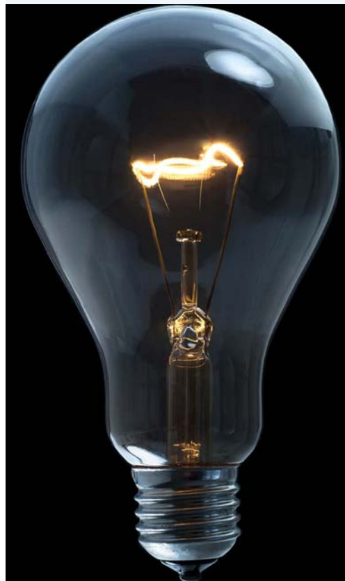
FIGURE 8.18 The glow of an incandescent light globe is caused by an electric current heating up a tungsten wire filament.
