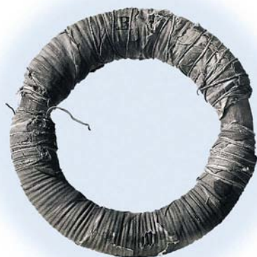
FIGURE 6.5 Photograph of the apparatus (two coils of insulated copper wire wound around an iron ring) that Faraday used to induce an electric current on 29 August 1831.
