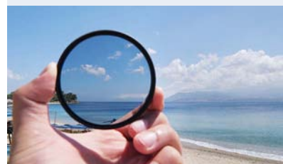
FIGURE 9.22 This polarising filter for a camera deepens the blue colour of the sky and sea.
