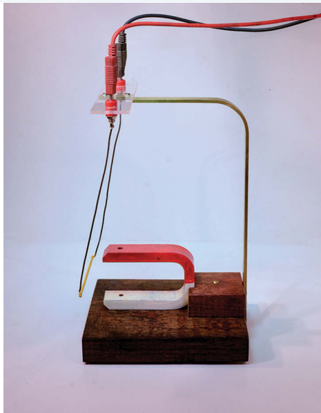
FIGURE 5.1 (a) A conductor is arranged as a swing, in a magnetic field (red is north). A current flows in the conductor and creates a magnetic field that interacts with the permanent magnetic field. (b) What change could have been made to the experiment to make the conductor swing in the opposite direction?
