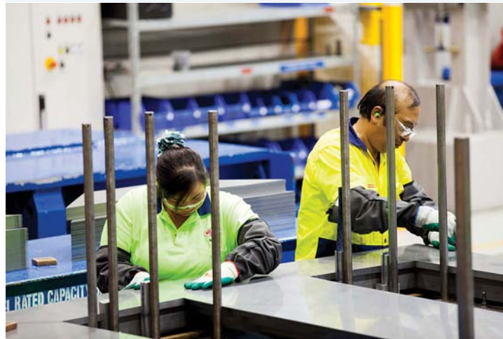
FIGURE 6.22 Workers assemble the laminated core at Wilson Transformers.
