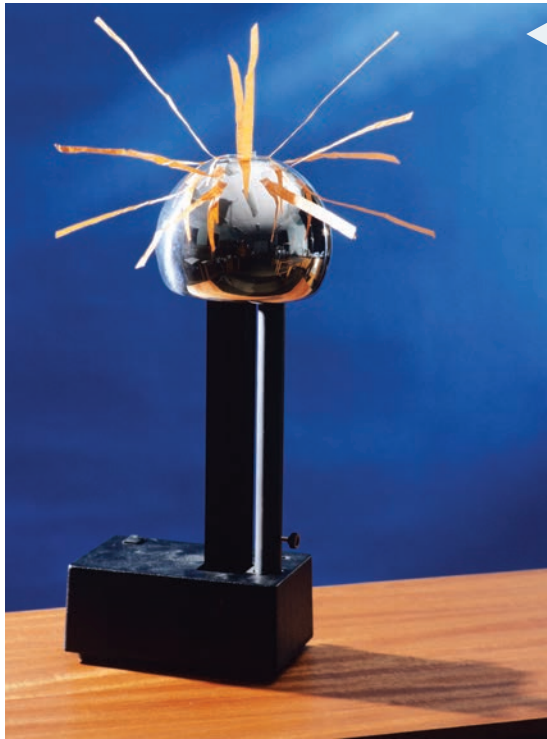
FIGURE 12.4 A van de Graaff generator. The paper attached to the dome becomes charged as it loses electrons to the positively charged dome.
