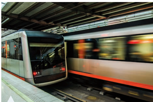
FIGURE 5.1 A train accelerates away from the platform. It is the friction force between the train's wheels and the rails that causes the acceleration.
