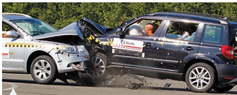
FIGURE 6.13 The crumple zone at the front of the car increases the time taken for the collision, thus reducing the force acting on the occupants.
