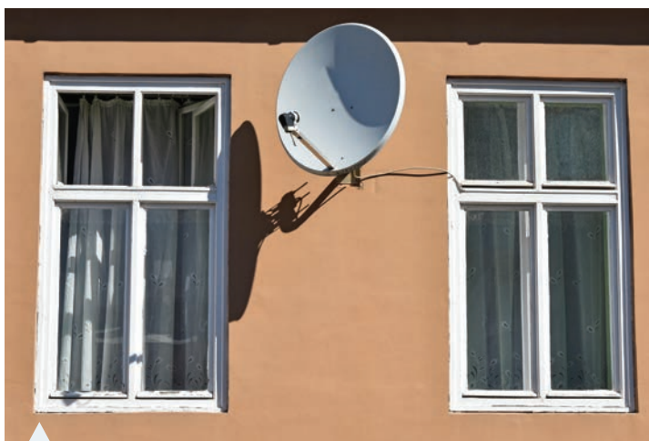
FIGURE 8.5 A typical parabolic satellite dish with the antenna placed at the focal point
