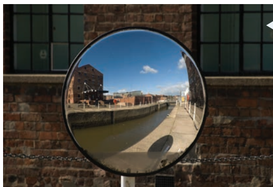
FIGURE 8.6 A convex mirror gives a wide field of view
