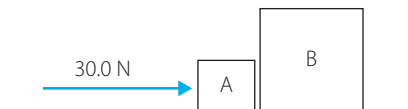
FIGURE 5.12 Two blocks on a frictionless surface are pushed to the right by a force of 30.0 N
