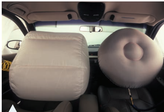
FIGURE 6.14 Front airbags spread the force applied to a passenger during a collision, as well as decreasing it.
