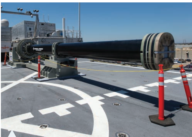
FIGURE 6.1 A rail gun uses the motor effect to fire a projectile at high speeds without using explosives.
