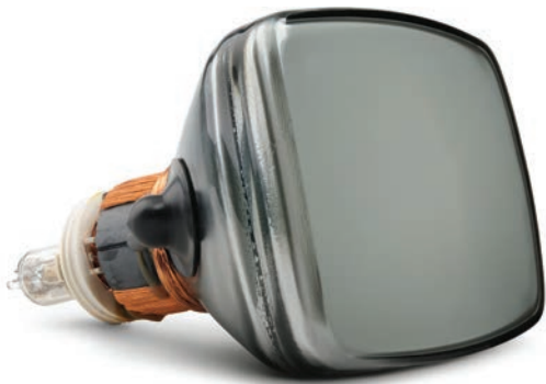
FIGURE 5.24 An old-style television picture tube
