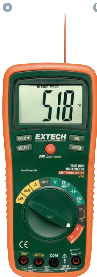
FIGURE 1.13 a A typical small digital multimeter; b A page from the user manual giving the precision on various scales. Note that instruction manuals often refer to 'accuracy' when the correct term is precision.
