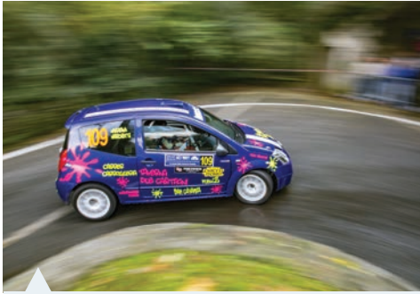
FIGURE 3.1 A car on a horizontal road turns as a result of the friction force applied to the tyres by the road.
