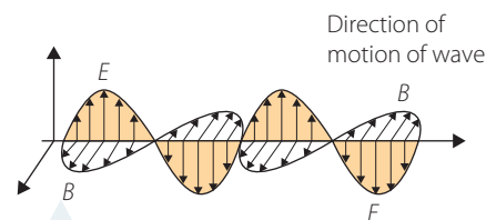
FIGURE 9.6 The electric and magnetic fields oscillate at right angles to each other, while the wave travels in the third dimension at right angles to both the electric and magnetic fields.
