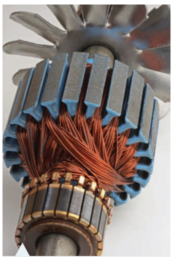
FIGURE 8.7 Most DC motors have multiple coils wound offset to each other.
