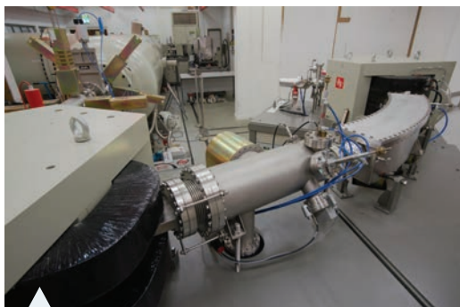
FIGURE 5.1 Part of the accelerator mass spectrometer in the Oxford Radiocarbon Accelerator Unit, used for dating samples of organic material.
