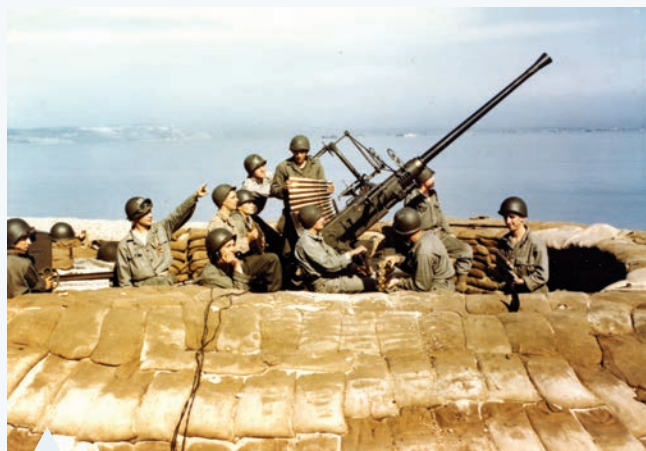
FIGURE 2.4 A 40 mm Bofors at-aircraft gun fires a shell with an initial velocity of around 1 \text{ km s}^{-1} .
