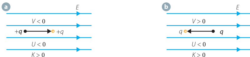
FIGURE 5.5 a A positively charged particle starting at rest will be accelerated in the direction of the field, to a point of lower potential. b A negatively charged particle starting at rest will be accelerated in the opposite direction to the field, to a point of higher potential. In both cases the particle gains kinetic energy and the particle–field system loses potential energy.
