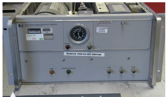
FIGURE 12.16 One of the atomic clocks used in the Hafele–Keating experiment
