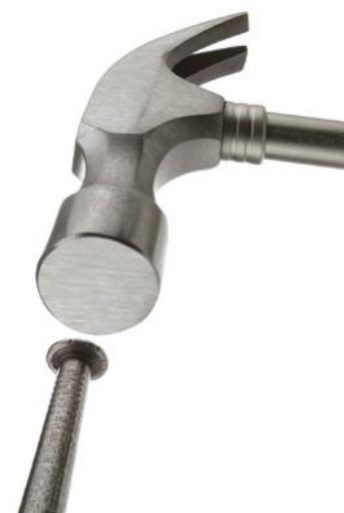
FIGURE 4.3.1 A hammer hitting a nail is a good example of an action–reaction pair and Newton's third law.
