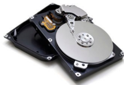
FIGURE 14.1.5 Ferromagnetic materials are used in many common applications, such as computer hard disk drives.
