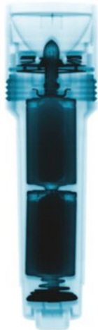
FIGURE 13.2.4 An X-ray image of the internal structure of a torch. The bulb and two batteries are clearly visible.
