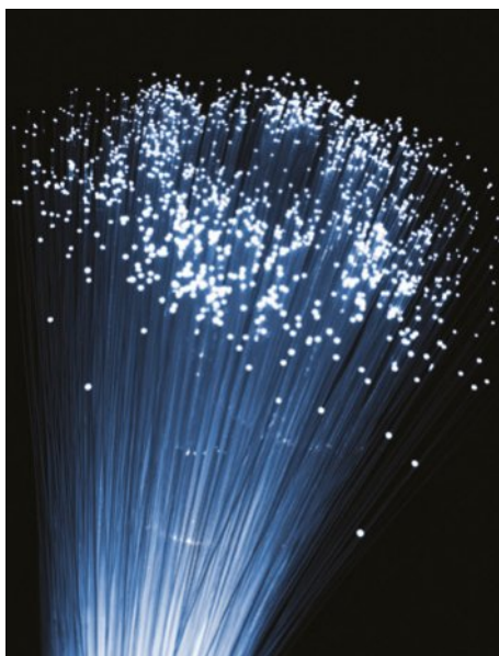
FIGURE 10.2.5 Optical fibres transmit light using total internal reflection.
