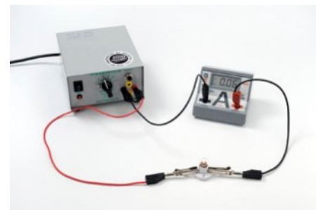
FIGURE 13.1.7 A digital ammeter (labelled with an A) measures current in a circuit.
