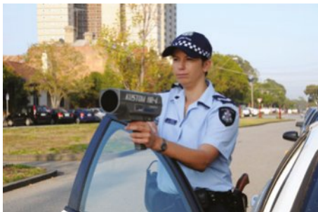
FIGURE 1.3.2 To avoid a systematic error, make sure that you are using measuring equipment correctly. Laser speed guns, for example, are held so that the aim is kept on a single target point for the duration of the reading.
