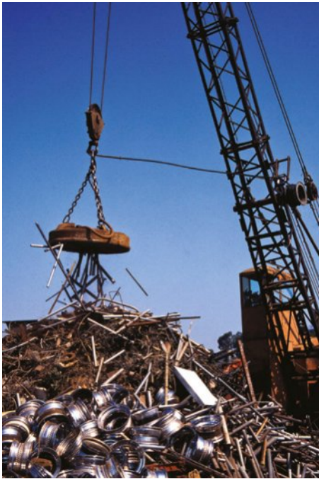
FIGURE 14.2.16 A large electromagnet being used to lift waste iron and steel at a scrapyard. Valuable metals such as these are separated and then recycled.
