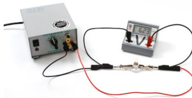
FIGURE 13.2.7 A voltmeter measures the voltage change (in this case, 6.23V) across a light globe.
