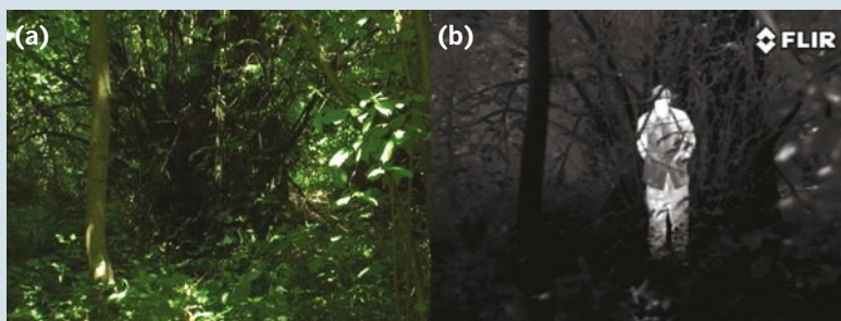
FIGURE 11.6.4 (a) The person standing behind the bush is difficult to see in normal light, but (b) they are warmer than the vegetation surrounding them and produce a stronger infrared emission, which a thermal imaging device is able to detect.
