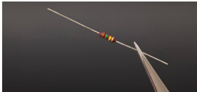
FIGURE 13.3.5 Common resistors are electrical devices with a known resistance. The coloured bands indicate the resistor's resistance and tolerance.
