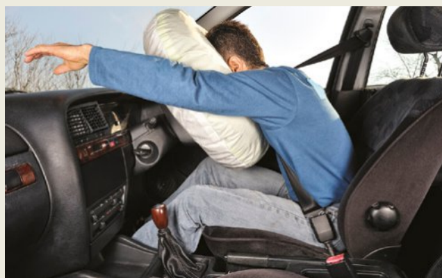
FIGURE 6.3.3 Airbags can prevent injuries by extending the period of time a person take to stop.
