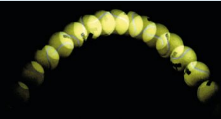
FIGURE 3.2.4 Adding together the vectors for the forward motion of the ball plus the downward motion of the weight create this parabola type shape.
