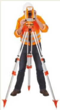
FIGURE 3.1.12 Surveying the land with a theodolite.
