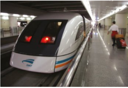
FIGURE 5.1.1 This magnetic levitation train in China rides 1 cm above the track, so the frictional forces are negligible. The train is propelled by a magnetic force to a cruising speed of about 430 \text{ km h}^{-1} .
