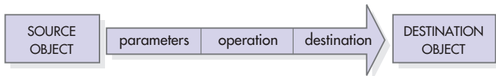
Figure 9.8 A message carries three vital pieces of information: its destination, an operation and the parameters.
