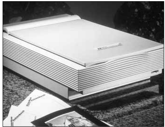
Figure 2.7 A scanner converts an image into a bit pattern which represents the picture.
