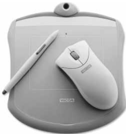
Figure 2.6 A digitising tablet can be used to 'draw' directly on a screen.
