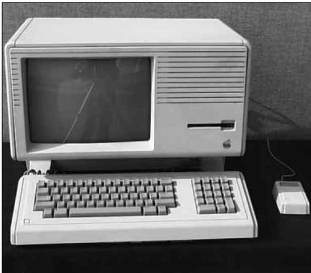
Figure 1.9 The Apple Lisa was the first commercial computer to use the GUI interface.
