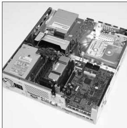
Figure 2.14 A hard disk drive is still a peripheral even though it may be housed inside the main system box of a computer.
