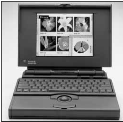
Figure 2.5 A trackball is really only a mouse on its back.
