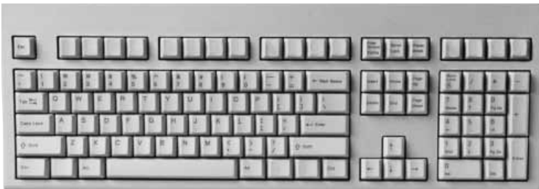
Figure 2.3 Computer keyboards are very much like a typewriter keyboard, but they usually contain more keys, which makes the keyboard more flexible.
