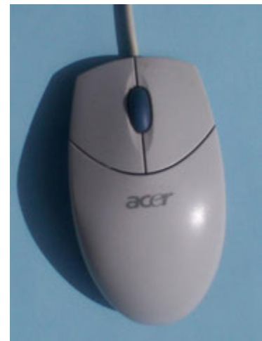
Fig 2.12 A typical mouse containing three buttons together with a scroll wheel.
