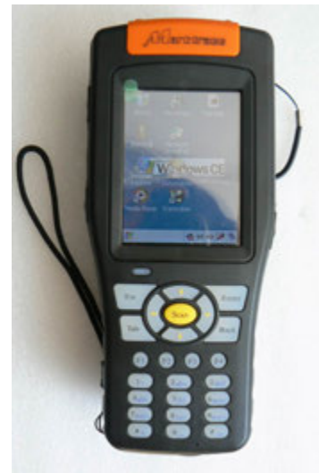
Fig 2.17 RFID reader integrated within a PDA.
