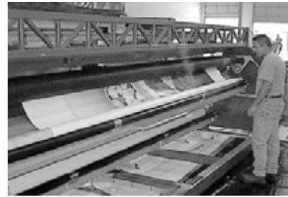
Fig 2.42 An inkjet printer capable of printing on various materials up to 6m wide.
