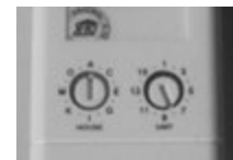
Fig 8.2 An X10 module set to house code A and unit code 8.
