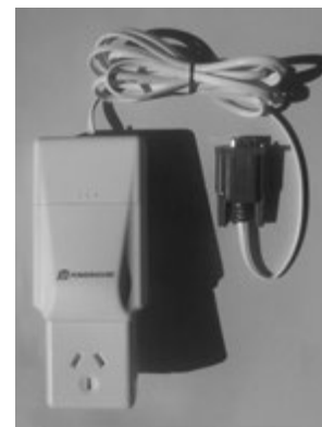
Fig 8.3 The CM11 computer interface module attaches to one of the computer's serial ports.
