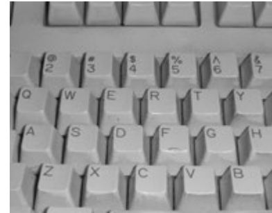
Fig 2.6 Section of a QWERTY keyboard. Note the staggered rows and standard size and shape of each key.
