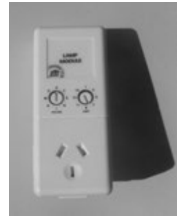
Fig 8.4 An X10 plug-in lamp module.
