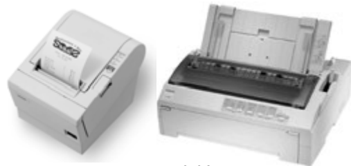
Fig 2.39 Epson's TM-T88 thermal receipt printer and FX-880 Impact dot matrix printer.
