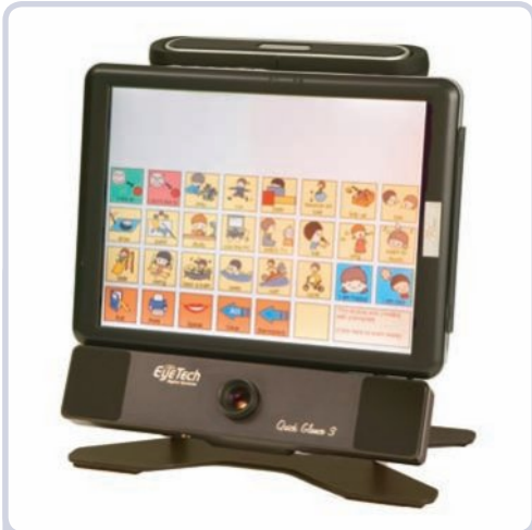
Figure 5.40 Computer system display intended to detect eye movement in a disabled user
