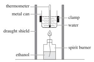
The ethanol in the spirit burner was burned to heat a known mass of water in the metal can. The student recorded the data obtained in the table below.
