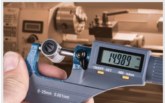
Digital micrometres and callipers measure in mm to 3 decimal places. Machinists require this level of accuracy when making intricate components, such as those designed by engineers for surgical instruments and engines of aircraft, ships and vehicles.
