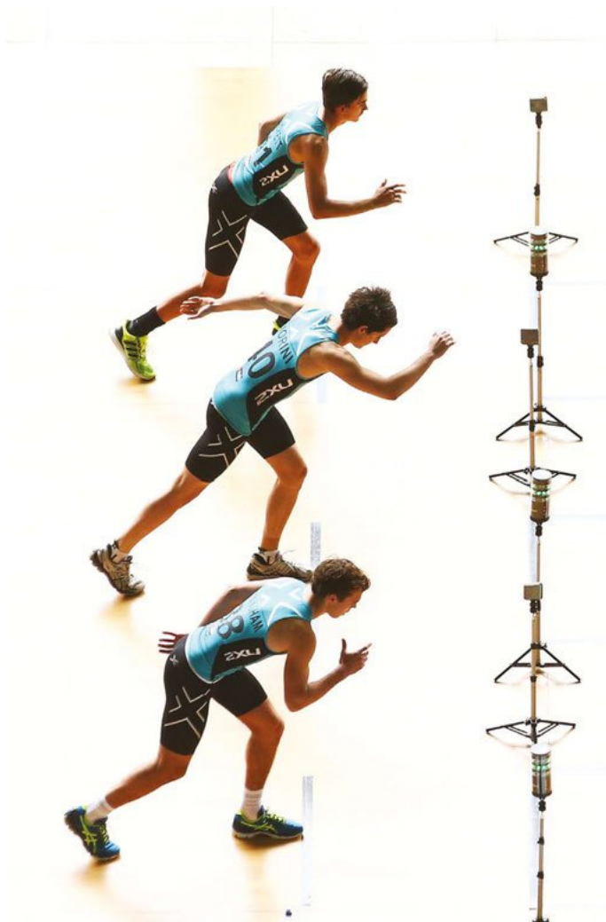
Figure 15.16 Timing gates measure speed at set intervals.
