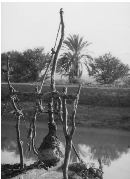
The shadouf, an ancient device for raising water, still in use along the Nile
