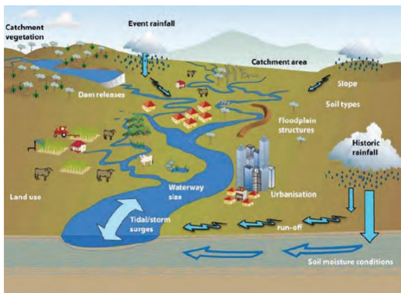
Figure 2.3.3n Rainfall is the most important factor in the onset of flooding, but there are many other contributing factors. When rain falls in a catchment, the amount of rainwater that reaches its rivers and streams depends on the characteristics of the catchment, particularly its size, shape and the land uses present. Some rainfall is ‘captured’ by soil and vegetation, and the remainder enters waterways as flow. River characteristics such as size and shape, the vegetation in and around the river, and the presence of structures in and adjacent to the waterway, all affect the level of water in the waterway.
