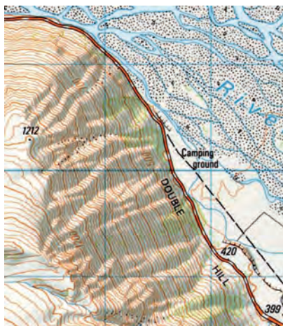
Figure 1.5b Shading on Lake Coleridge topographic map extract. Shading creates a three-dimensional visual effect.
