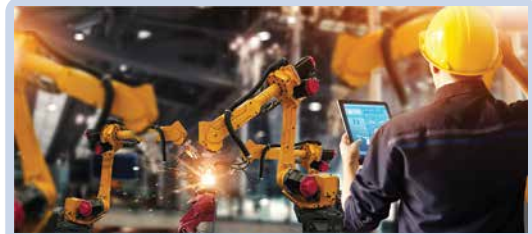
Programs that manipulate a robot's arm include circle equations. Working in 2D: with the lower arm secured at its base, the joint can move in a semicircle; each point on this semicircle can be the centre of a circular path that the hand can follow.
