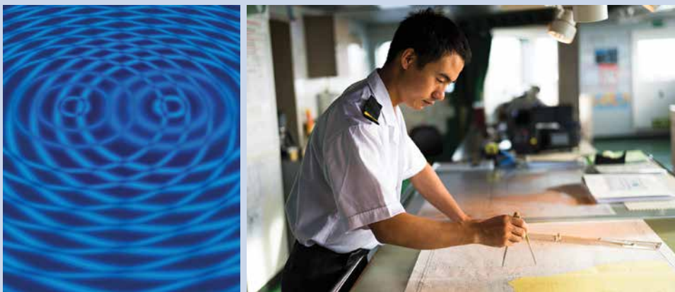
Two signal pulses emitted simultaneously will spread in overlapping concentric circles. All circle intersection points with the same difference in distance (or time) from the centres form a hyperbola shape. Using signal time differences and hyperbolic charts, navigators can locate a ship's position more reliably than using GPS.
