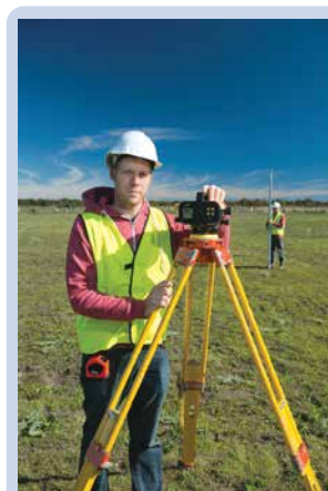
Land surveyors measure the horizontal and vertical distance between two locations of different altitudes. The straight line distance of the slope, which forms a hypotenuse, is calculated using Pythagoras' theorem.
