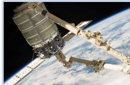
The International Space Station has a 16.94 m robotic arm with four segments that's used on spacewalks, and capturing and releasing visiting spacecraft. Trigonometry is used to calculate the required angle between segments for grabbing specific spacecraft.
