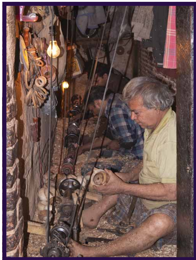
An Indian sweat shop worker making wooden curtain rings on primitive lathes in a very small windowless room
