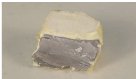
Figure 7.36 A piece of sodium metal which has been cut by a knife. It is shiny on the inside and dull on the outside.
