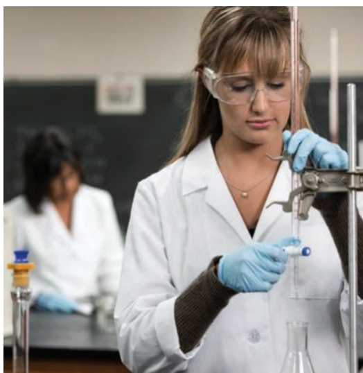
Figure 1.8 A burette in a retort stand being used to perform a titration.
