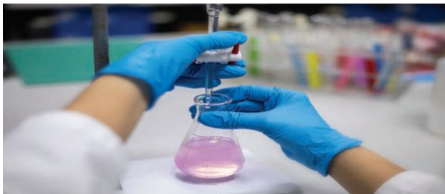
Figure 1.15 Example of titration set-up for Part 4 of this experiment with pink phenolphthalein indicating that end point is reached
