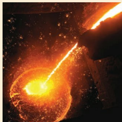
Figure 8.8 Molten iron spews out of a blast furnace where iron ores are reacted with carbon to form pure iron metal.
