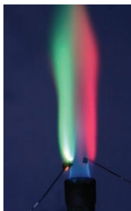
Figure 7.26 A copper compound burning with a green flame and a lithium compound burning with a red flame
