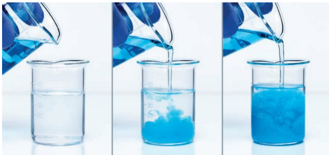
Figure 8.13 A blue solution is added to a colourless solution to form a blue precipitate in a colourless solution.
