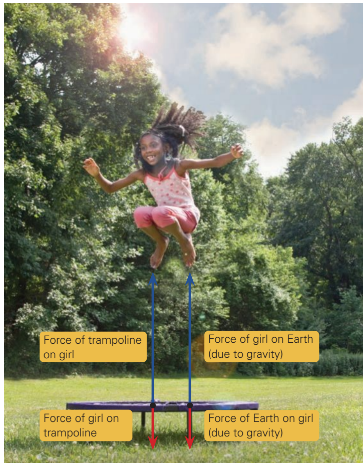
Figure 6.37 As a person lands on a trampoline, they exert a force downwards on the mat when in contact with the mat. The mat then pushes them back up with an equal but opposite force. This causes the person to slow down and stop, then bounce back into the air.
