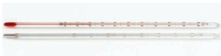
Figure 1.15 The liquid in the glass thermometer shown uses the measurement unit Celsius ( ^{\circ}\text{C} ). The thermometer with a red coloured liquid is modern and uses alcohol, while the thermometer with the grey coloured liquid is mercury. Why might mercury thermometers have been phased out of production?
