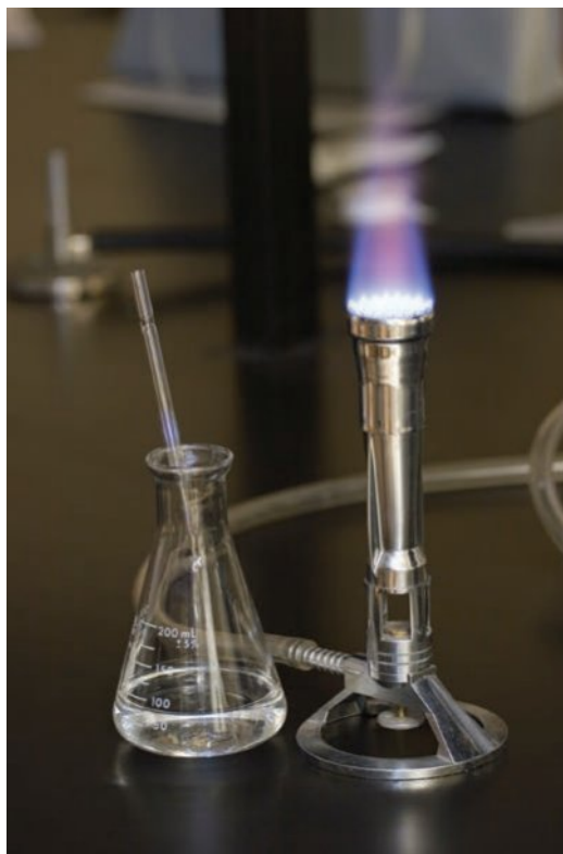
Figure 1.5 The Bunsen burner blue flame is produced when the airhole is fully open. It allows oxygen from the air to mix with the gas in the barrel producing a hotter flame.
