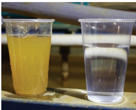
Figure 8.12 Samples of water with flocculant added (left) and the resulting water after treatment (right)
