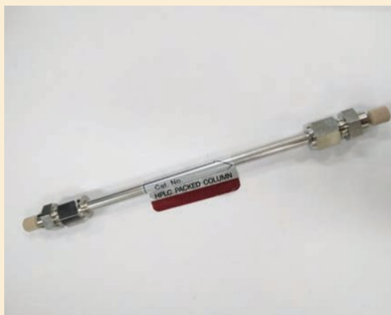
Figure 8.27 A densely packed HPLC column
