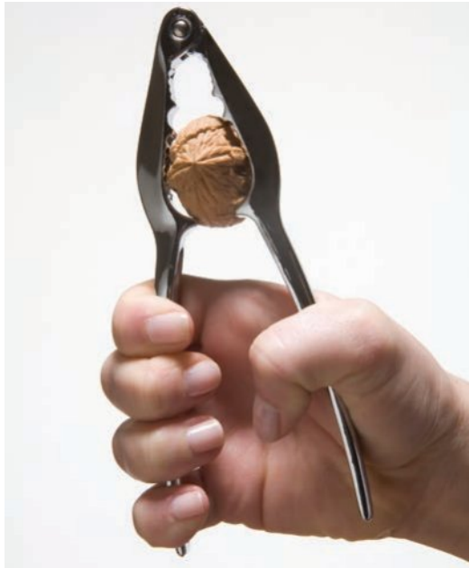
Figure 6.1 A nutcracker is an example of a lever.
