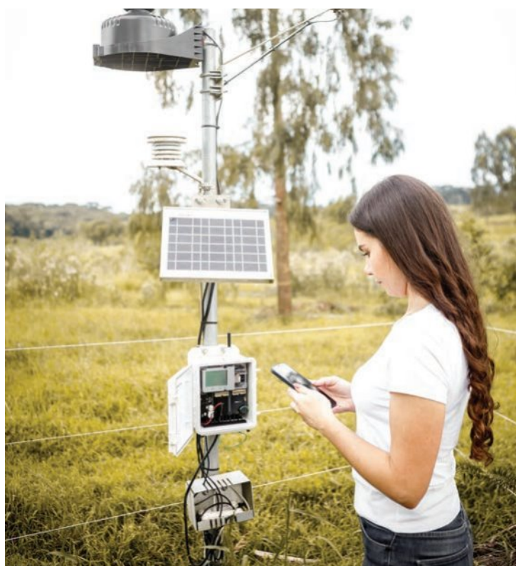
Figure 1.14 Many weather monitoring systems employ data loggers.
