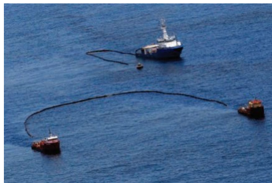
Figure 8.42 A boom is an inflatable barrier used to contain an oil spill.
