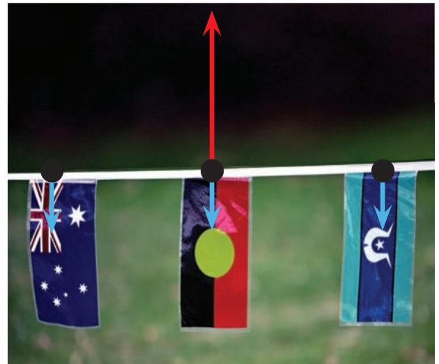
Figure 5.4 The tension in the tape pulling up (red) is equal to the sum of the pull down (blue) forces of the three flags due to gravity.
