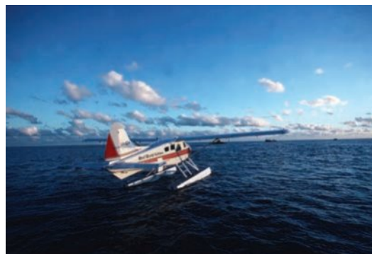
Figure 5.27 Seaplanes use floats instead of wheels to land on water.
