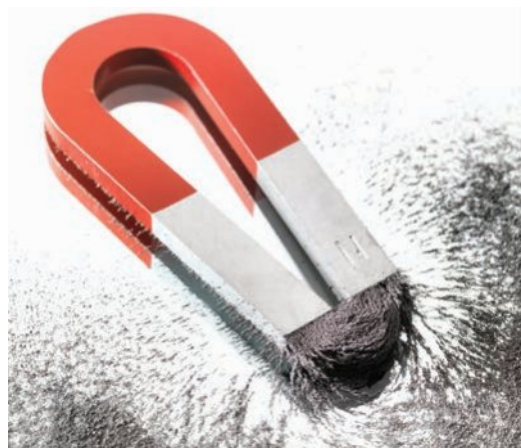
Figure 8.11 A magnet can be used to separate magnetic substances from non-magnetic substances.
