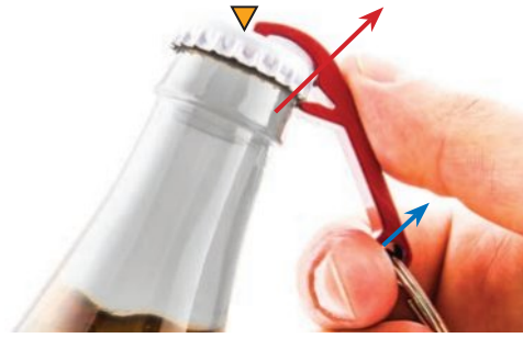
Figure 6.3 A bottle opener is a class 2 lever. The fulcrum (shown by the orange triangle) rests on the cap and the effort force is applied to the handle. This results in a large load force on the edge of the cap, which opens the bottle. It would otherwise be difficult to open the bottle with our bare hands.
