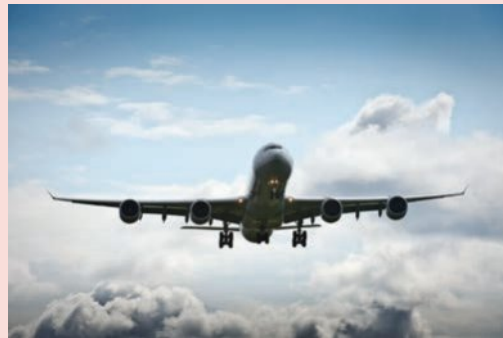
Figure 5.31 The Airbus A340 laminar-flow demonstrator 'BLADE' aircraft in flight for testing
