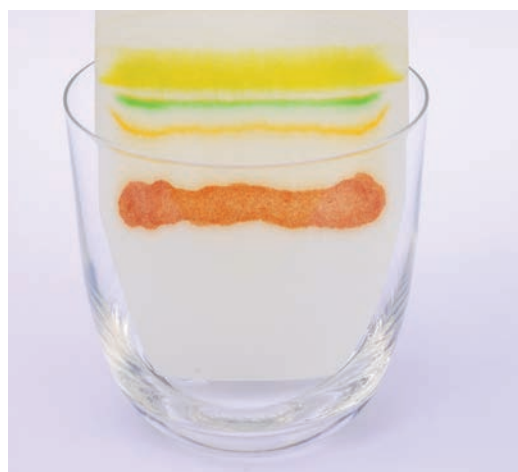
Figure 8.25 Paper chromatography can be used to separate vegetable pigments, where the yellow component is most soluble and the orange is the least soluble in the solvent.
