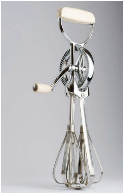
Figure 6.29 A manual egg beater. The handle turns the large gear, which in turn spins smaller gears that cause the beaters to spin fast.
