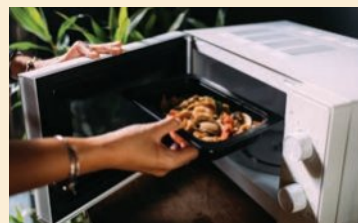
Figure 7.10 Microwave ovens work by causing the water particles in food to vibrate and heat up.
