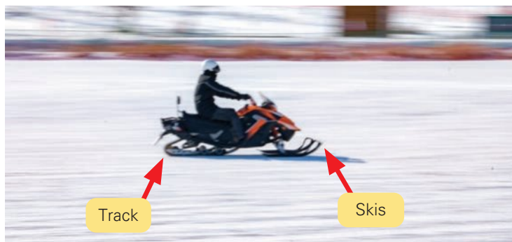
Figure 5.57 Snowmobiles use skis and a track instead of wheels.
