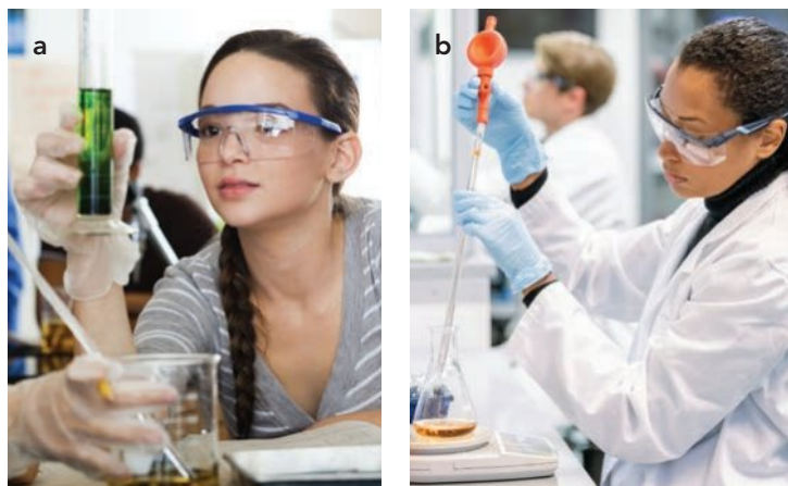
Figure 1.13 (a) A measuring cylinder and (b) a scientist using a glass pipette for dispensing a volume of liquid
