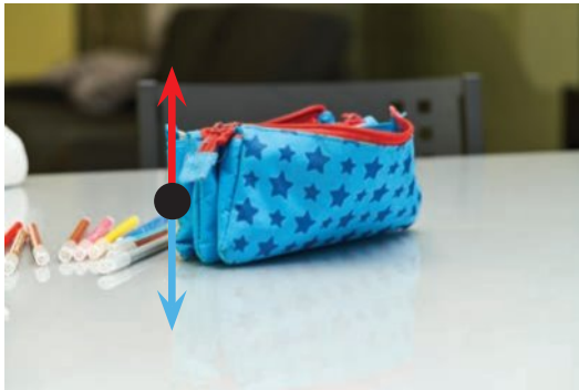
Figure 5.8 The weight force of the pencil case (blue) is pulling down towards Earth due to gravity. This is balanced by the normal force of the desk pushing back at it (red).
