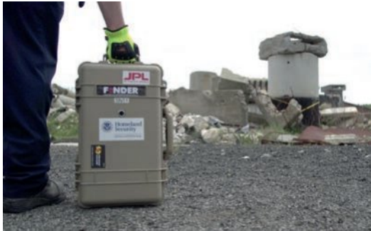
Figure 4.70 The FINDER device uses microwave radar sensors to remotely detect heartbeats and locate survivors.
