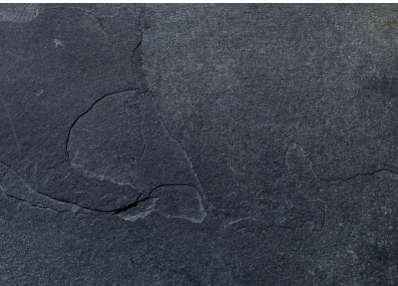
Figure 5.22 Slate is a metamorphic rock formed when mudstone is subjected to high pressure and temperature.
