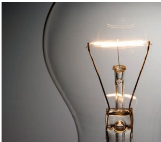
Figure 6.46 A filament light bulb emits light energy but also thermal energy as waste.
