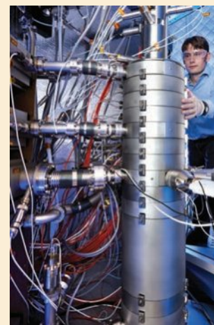
Figure 7.8 This transmission electron microscope in the USA can observe atoms.
