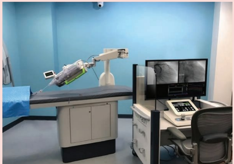
Figure 3.48 Using robots to perform angioplasties is not only safer for medical staff but also more accurate.
