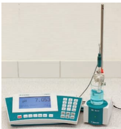
Figure 1.15 By using a pH meter instead of pH paper, more accurate and precise pH measurements can be made.
