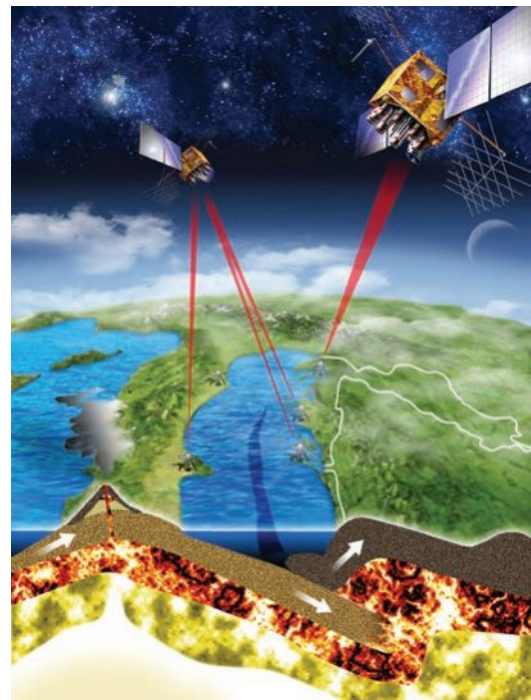
Figure 4.64 GPS is used to measure position and therefore the rate of movement of tectonic plates.
