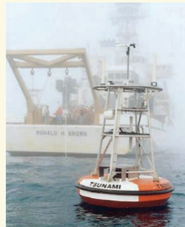
Figure 4.67 DART® (Deep-ocean Assessment and Reporting of Tsunamis) real-time tsunami monitoring systems are positioned throughout the ocean and play a critical role in forecasting tsunamis.
