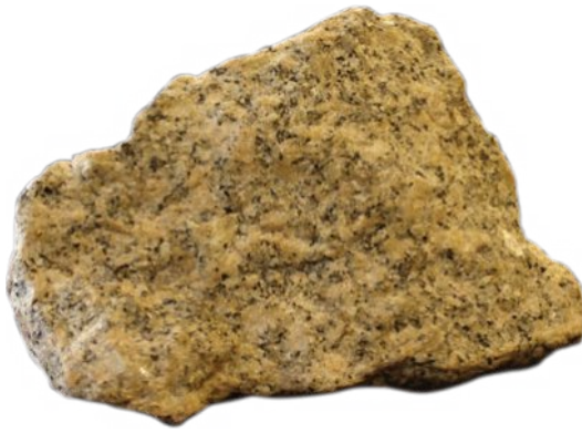
Figure 5.5 Granite is an igneous rock. It is usually made up of four minerals. The large crystal size in the rock indicates that the rock cooled slowly, probably underground.
