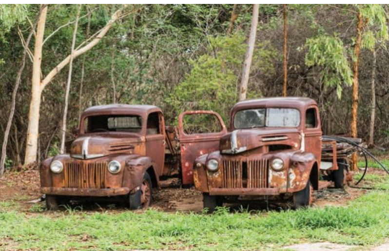
Figure 8.16 Iron metal corrodes to form brown iron oxide after years of exposure to oxygen and water.
