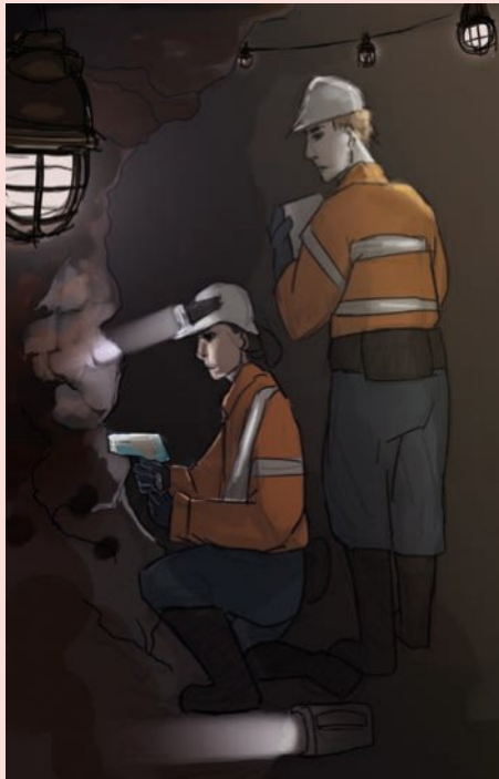
Figure 5.88 Miners can use a PMI gun to determine the composition of a rock.
