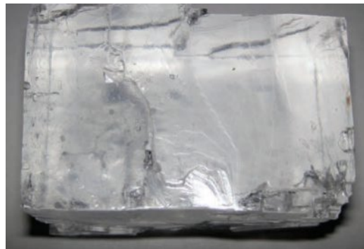
Figure 5.43 Rock salt is a sedimentary rock made of halite, a mineral composed of sodium chloride, NaCl.
