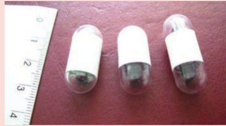
Figure 3.80 Camera capsules used to examine the oesophagus (left), small intestine (middle) and large intestine (right)
