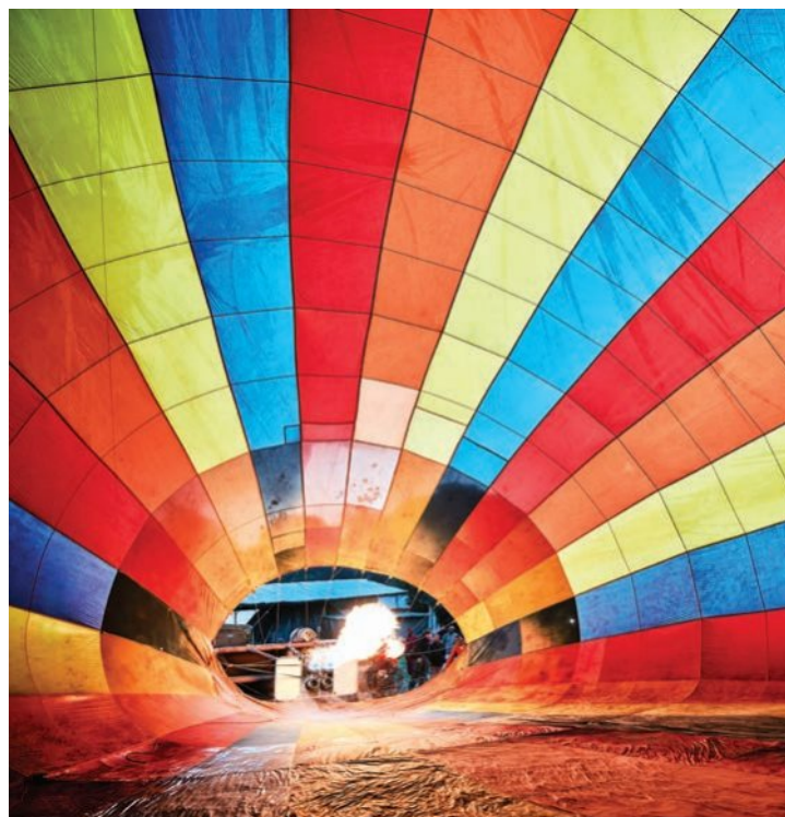
Figure 8.4 When the air inside a hot-air balloon is heated, the atoms in the heated air gain energy, move faster and move away from one another, therefore taking up more space. This is an example of a physical change occurring and it results in the air being less dense on the inside of the balloon, so the balloon rises.
