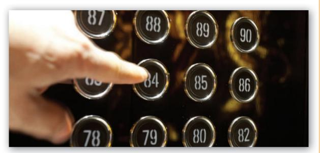
The electronic controller for a building lift runs an algorithm that delivers people to their destination based on which buttons are pressed both inside the lift car and in lift waiting areas. The algorithm must accept the requests (inputs: which buttons are pressed) and deliver a result (output: the action of the lift car) so that passengers travel to where they want to go in an efficient manner. A basic algorithm for a lift is as follows:
