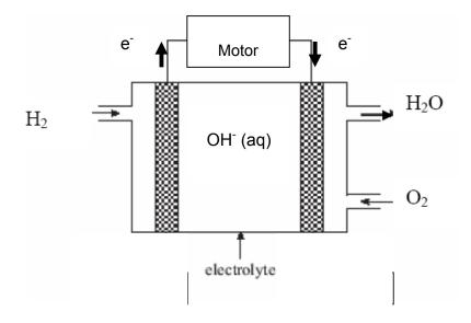
The fuel cell consists of two sections: hydrogen gas is pumped through one half and oxygen gas the other. The two halves are joined and an alkaline electrolyte such as KOH passes through the middle. The electrodes consist of a porous nickel alloy mesh.
