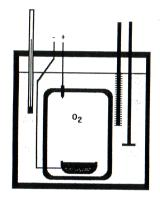
In one experiment, a current of 2.50 A was passed through the electric heater of a bomb calorimeter for 60.0 seconds at a voltage of 5.50V causing a temperature rise of 0.529°C.
