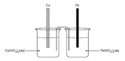
The solutions are connected to each other with a salt bridge consisting of an inverted U-tube containing an appropriate electrolyte.
